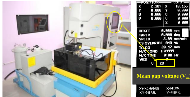
Fig. 1 (a) Machine tool (b) Integrated computer displaying mean gap voltage
