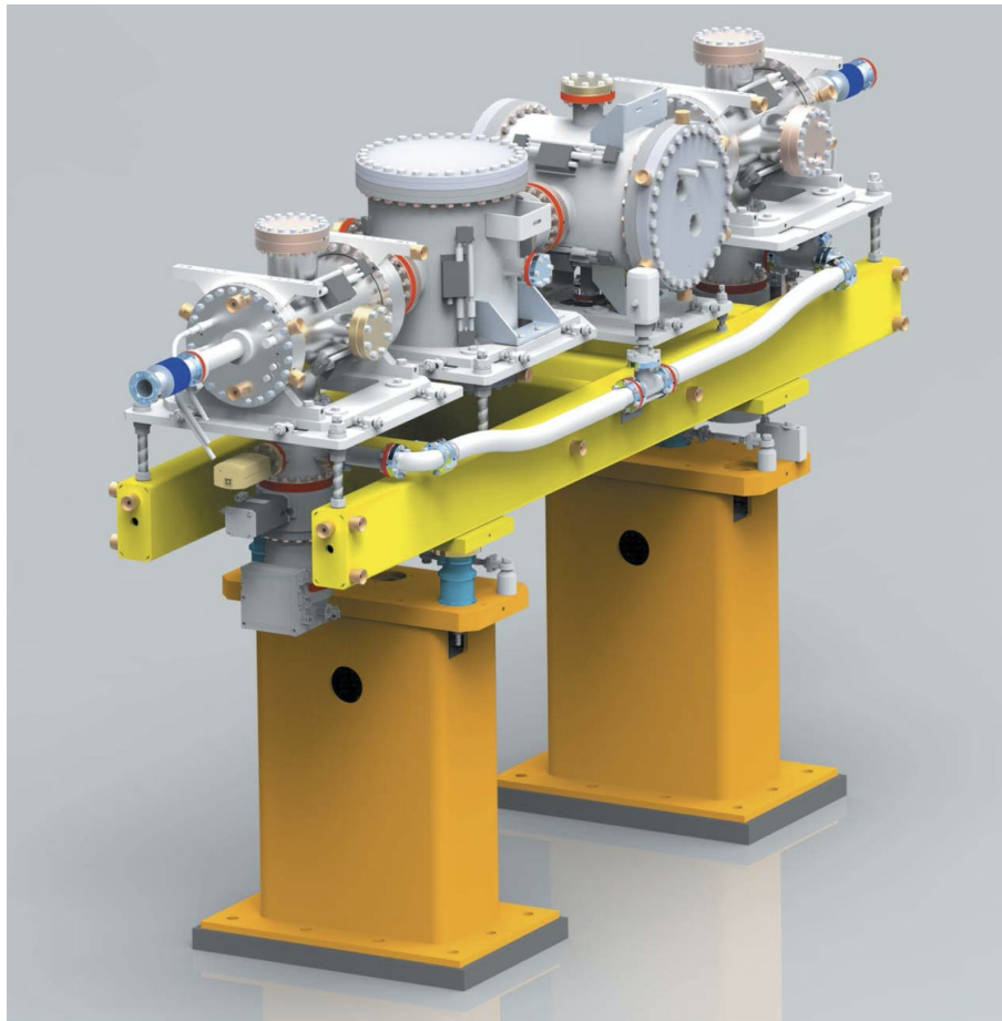
Figure 6.64.: CAD rendering of the XGM used at the European XFEL. Figure from [263].
