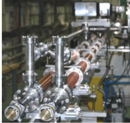
Figure 5.53.: 30 GHz SLED2 pulse-compressor in CTF3.
