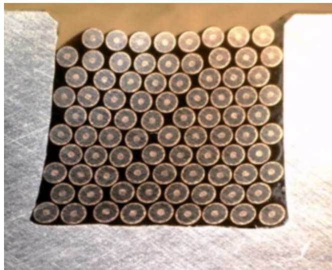
Figure 6.17.: Cut through of undulator winding, showing the winding stack.
