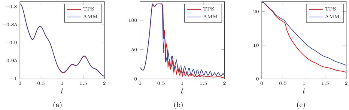
FIGURE 3. Experiment of Section 4.1: comparison of the results obtained with TPS and AMM for  $\ell = 6$ ,  $k = h_6/100$ , and  $\varepsilon = h_6/100$ . (a) Evolution of the average magnetisation  $\langle m_3 \rangle$ . (b) Evolution of the  $W^{1,\infty}$ -seminorm. (c) Evolution of the total energy.
