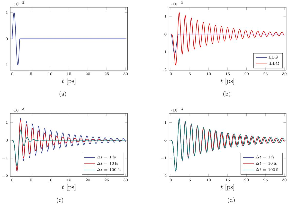
FIGURE 5. Experiment of Section 4.2: (a) Plot of the function  $t \mapsto F(t)$  which modulates the amplitude of the pulse field. (b) Evolution of  $\langle m_3 \rangle$  for LLG and iLLG computed with TPS for  $\Delta t = 1$  fs. (c) Evolution of  $\langle m_3 \rangle$  computed with TPS for different time-step sizes. (d) Evolution of  $\langle m_3 \rangle$  computed with AMM for different time-step sizes.
