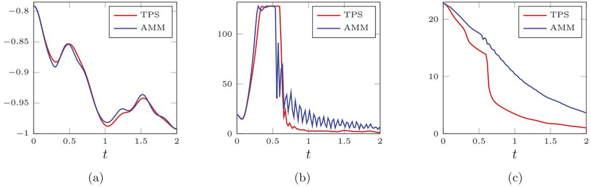
FIGURE 2. Experiment of Section 4.1: comparison of the results obtained with TPS and AMM for  $\ell = 6$ ,  $k = h_6/10$ , and  $\varepsilon = h_6/10$ . (a) Evolution of the average magnetisation  $\langle m_3 \rangle$ . (b) Evolution of the  $W^{1,\infty}$ -seminorm. (c) Evolution of the total energy.
