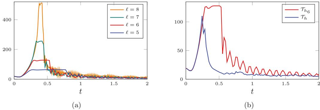
FIGURE 4. Experiment of Section 4.1: evolution of the  $W^{1,\infty}$ -seminorm obtained with AMM for different mesh resolutions (a) and different symmetry properties (b). (a)  $W^{1,\infty}$ -seminorm for  $\ell = 5, 6, 7, 8$ . (b)  $W^{1,\infty}$ -seminorm for  $\mathcal{T}_{h_6}$  and  $\mathcal{T}_h$ .
