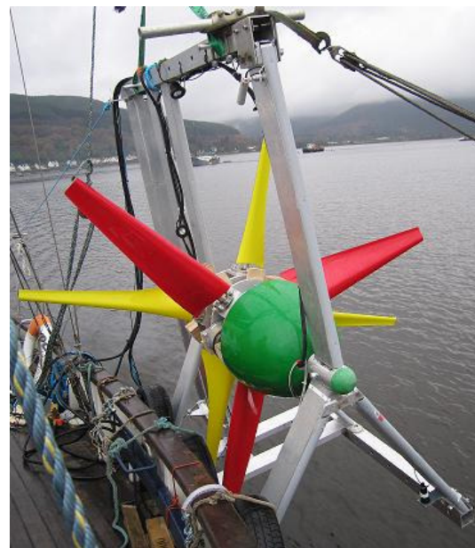
Figure 1: 2.5m diameter contra-rotating Marine Turbine (CoRMaT)
