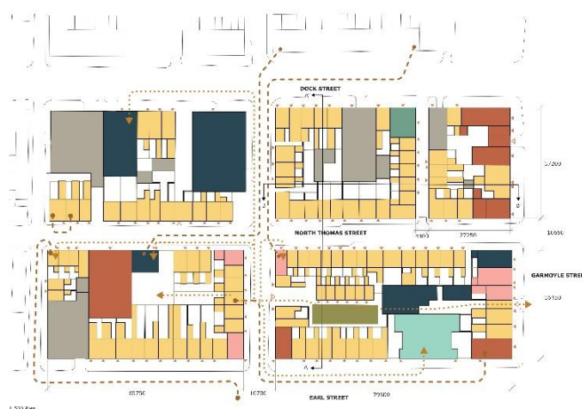
Figure 2. Plan analysis into the four blocks after the drawing of the axonometric. Uses, entrances, green space, routes and shortcuts are highlighted.
