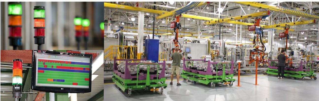
*Figure 3. Implement sign boards, colour code, and non-verbal communication at a workplace. (photos: <https://sullivanlehdesigns.com/clients/andonix/andon-cord/>, <https://www.assemblymag.com/articles/94443-signal-tower-data-collection-increases-productivity>, <https://www.americanexpress.com/en-us/business/trends-and-insights/articles/why-made-in-the-usa-is-making-a-comeback/> )*
