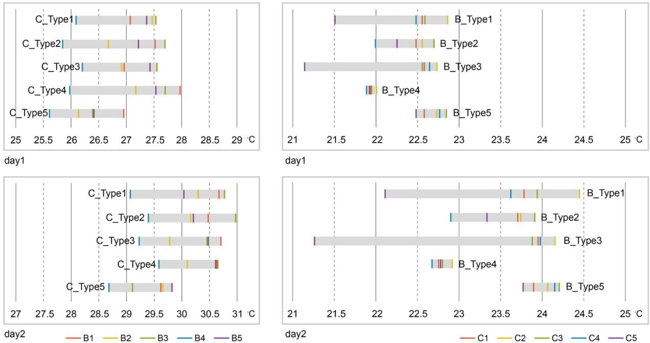
**Figure 4.** Maximum daytime outdoor temperature aggregated for context types (left), and average daytime indoor temperature aggregated for building types (right)
