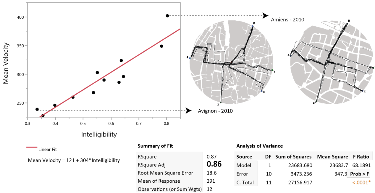
Figure 4. Linear fit between the measure of mean velocity (30 paths) and intelligibility per city and period (12 maps). The maps of Avignon and Amiens in 2010 illustrate a respectively low and high intelligible structure.
