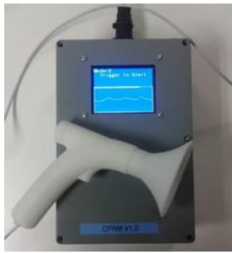
Figure 1 - The contactless portable respiratory rate monitor (CPRM); interface unit.
