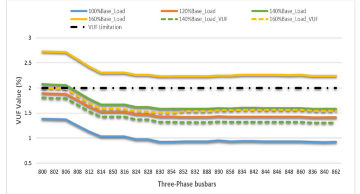
Fig. 7. VUF results comparison between with and without voltage unbalanced constraint in different level of unbalanced load
