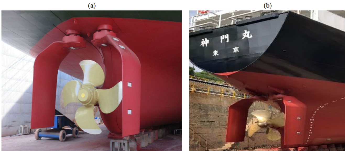
Fig. 1 Installed Gate Rudder System in actual ship (a) MV Shigenobu (b) Shinmon Maru
