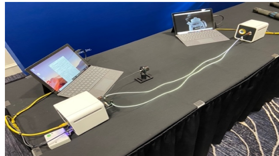
Figure 3. Experimental system of dual laser LiFi system with emissive fiber shown.
