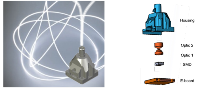
Figure 2. Image and schematic of the fiber coupled SMD light source showing SMD on electronic board, collimating and focusing optics, and housing.
