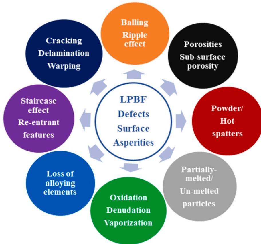
Fig. 14. List of various metallurgical defects and surface asperities emerge during LPBF process.
