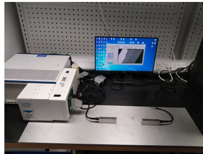
Fig. 6. Experimental set up showing the two linear arrays on top of the 1\text{m} \times 30\text{cm} \times 10\text{mm} aluminium plate and the array controller.
