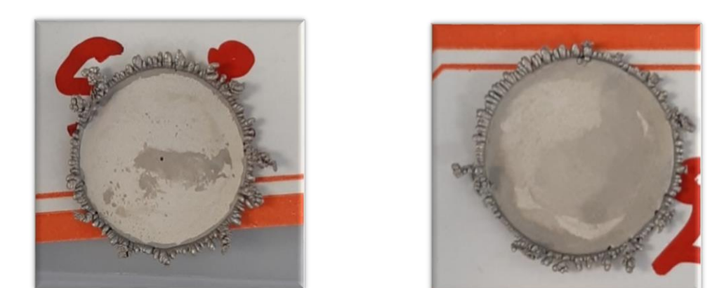
The quality of the deposits developed by the use of the UoS-prepared electrolyte was “higher” while, the deposits prepared by the use of the company’s electrolyte sample presented higher dendritic growth. Investigations to determine the reasons for these observations are ongoing.
