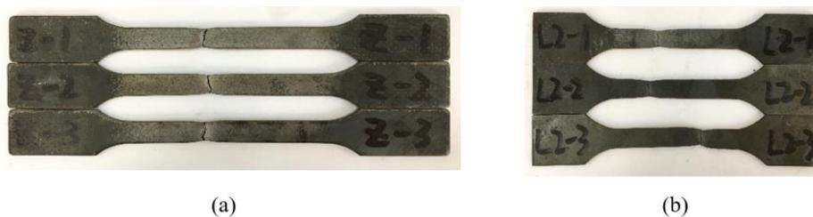
Fig. 5. Photos of the coupons of: (a) the column, and (b) Beam II
