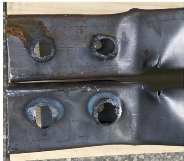
(b) bottom view of the cracked flanges
