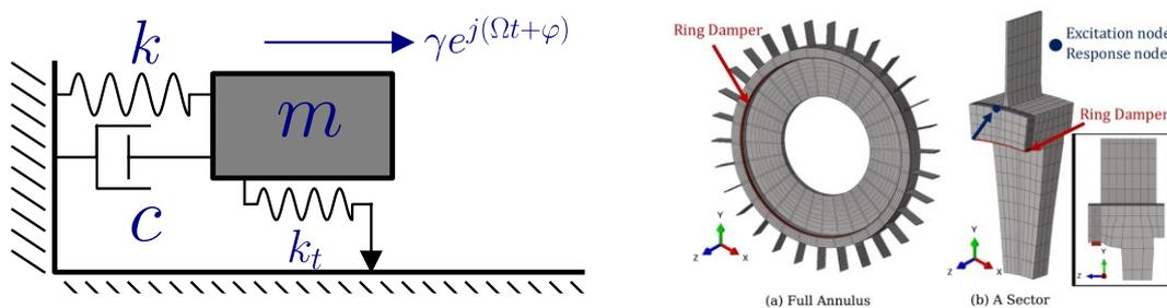
**Figure 1** 1 DOF System (left) and full-scale blisk with friction ring damper (right) [4]
