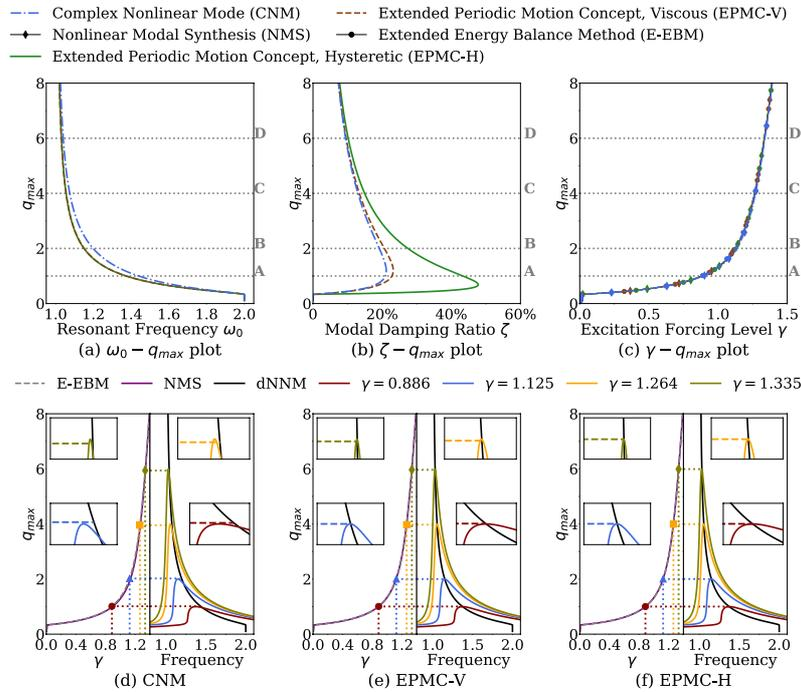
**Figure 2** Testcase I: (a, b, c) Numerical results from the damped nonlinear normal mode within a range of modal amplitude; (d, e, f) Using nonlinear forced response to validate frequency -modal amplitude curves and force level-modal amplitude curves [4].
