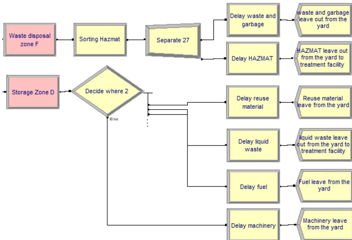
Figure 17. Segregation module in the zone D
