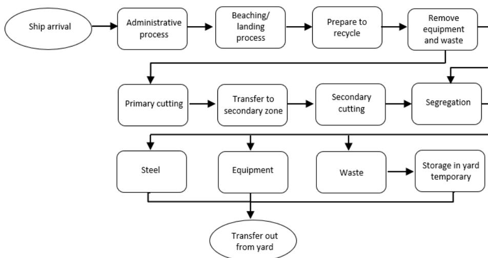
Figure 5. Simplified ship recycling process flow for observed yard in Indonesia
