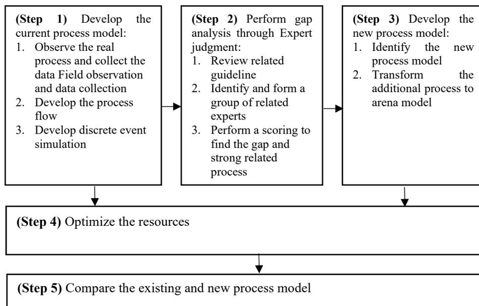
Figure 1. Methodology for improvement process model in ship recycling yard using discrete event simulation and expert judgment in terms of efficiency
