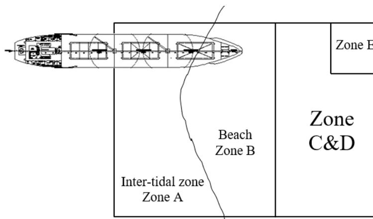
Figure 2. Current layout of Case Study Ship Recycling Yard
