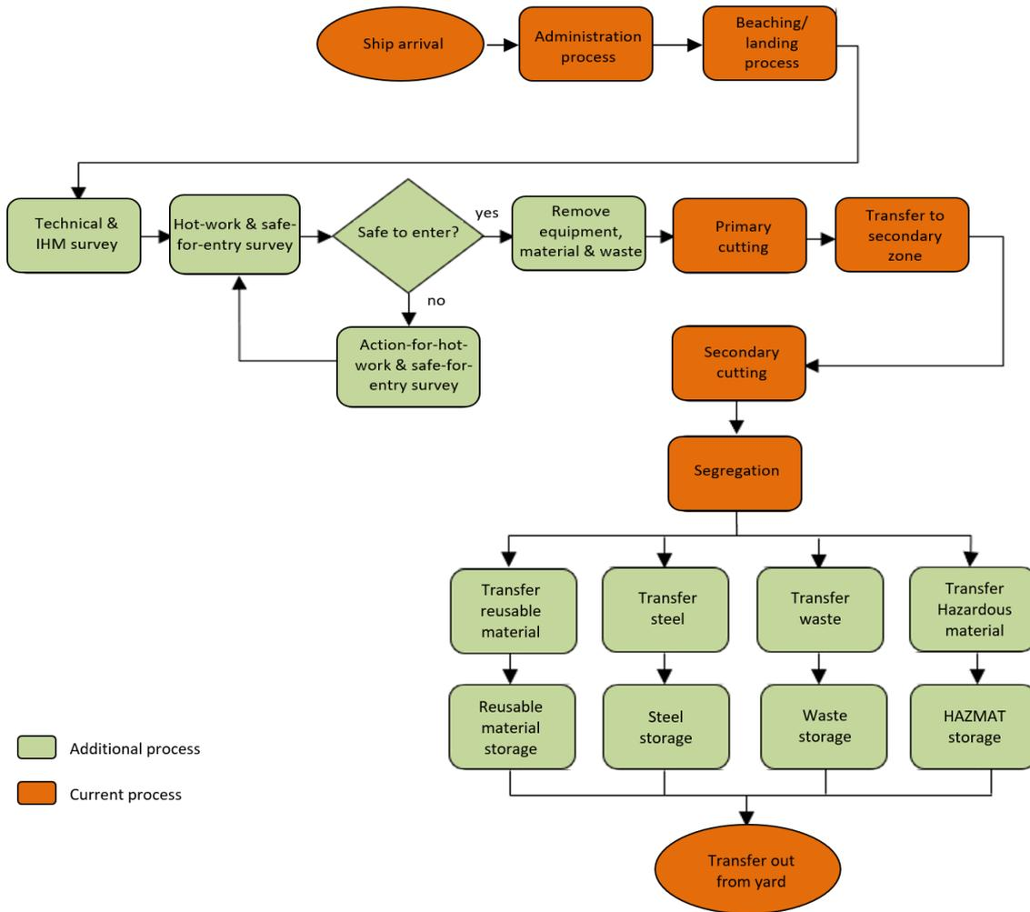
Figure 14. The new process models.
