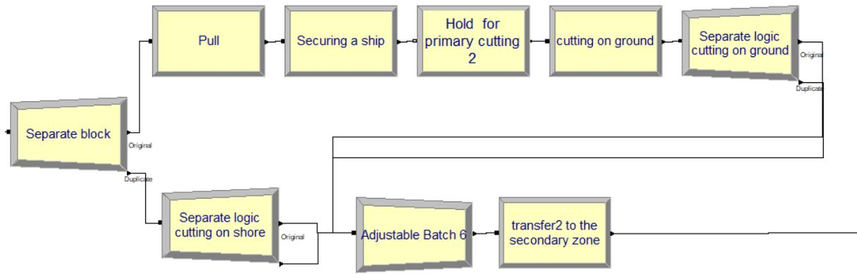
Figure 10. Primary cutting model in ARENA simulation
