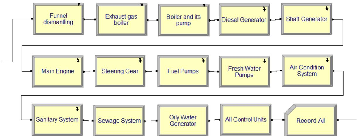
Figure 12. Sub model of machinery removal model in ARENA simulation
