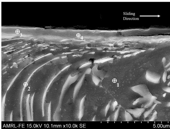
Fig. 17. Carbide/oxide surface layer and EDS points on 500C 6 kg disc. [x10000 – nital].
