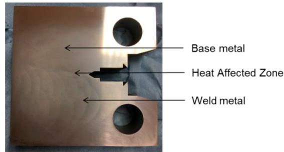
Fig. 2. C(T) specimen extracted from the welded slice
