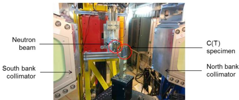
Fig. 3. Neutron diffraction experimental set up on Engin-X
