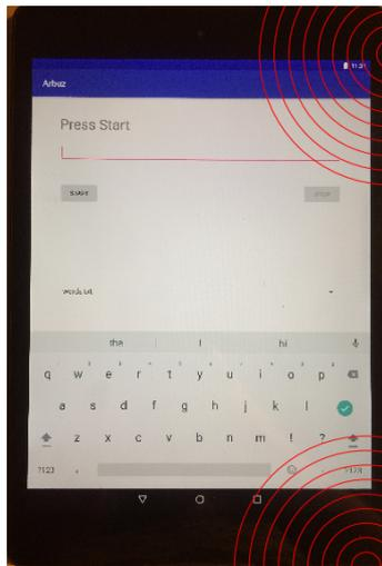
Figure 5: The location of the two Nexus 9 microphones, where the length between the subsequent radii is the distance travelled by a sound wave through air during one sampling period.
