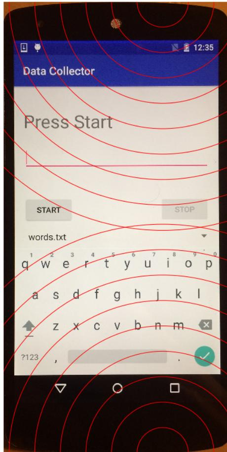
Figure 3: The location of the two Nexus 5 microphones, where the length between the subsequent radiuses is the distance traveled by a soundwave through air during one sampling period.
