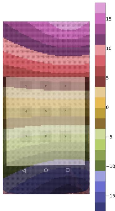
Figure 6: The location of the two Nexus 5 microphones, where the length between the radii around each microphone is the distance travelled by a soundwave during one sampling period.
