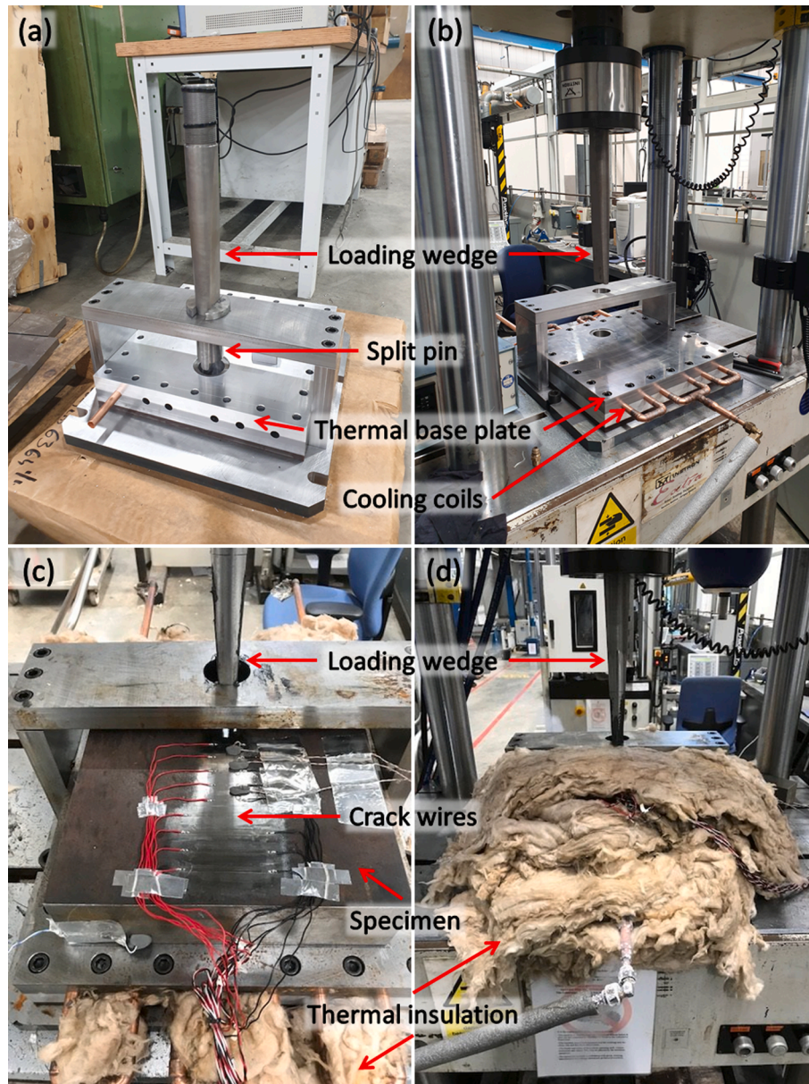
Fig. 3. Experimental set up of CCA tests showing: (a) the test rig assembly, (b) the fully assembled test rig on the machine, (c) the specimen is placed in the test rig and instrumented, (d) during the test.
