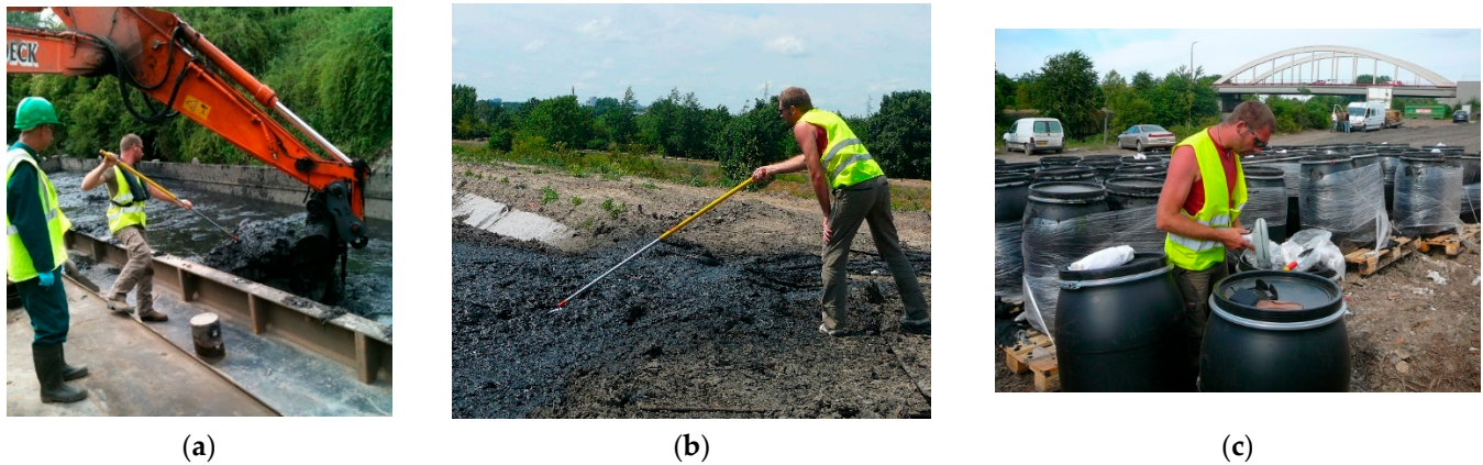
Figure 1. Sampling and analysis during sediment loading and unloading: (a) Sampling a barge load with a small trowel mounted on a telescopic handle; (b) Sampling from an unconsolidated lagoon; (c) checking lots before sending to a processing test.
