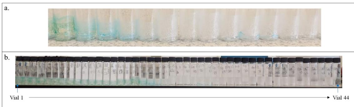
**Figure 5.** (a) Close-up of a few dried filtrate vials showing the presence of the precipitated material. (b) Collected filtrate vials from experiment 15 showing gradual blue dye impurity removal from the system.
