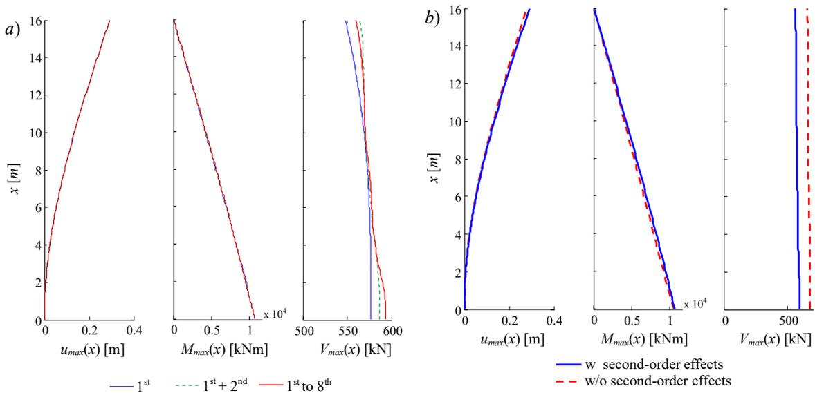
467 Fig. 9. Average seismic response of case study 2: a) modal contributions to the displacements,
