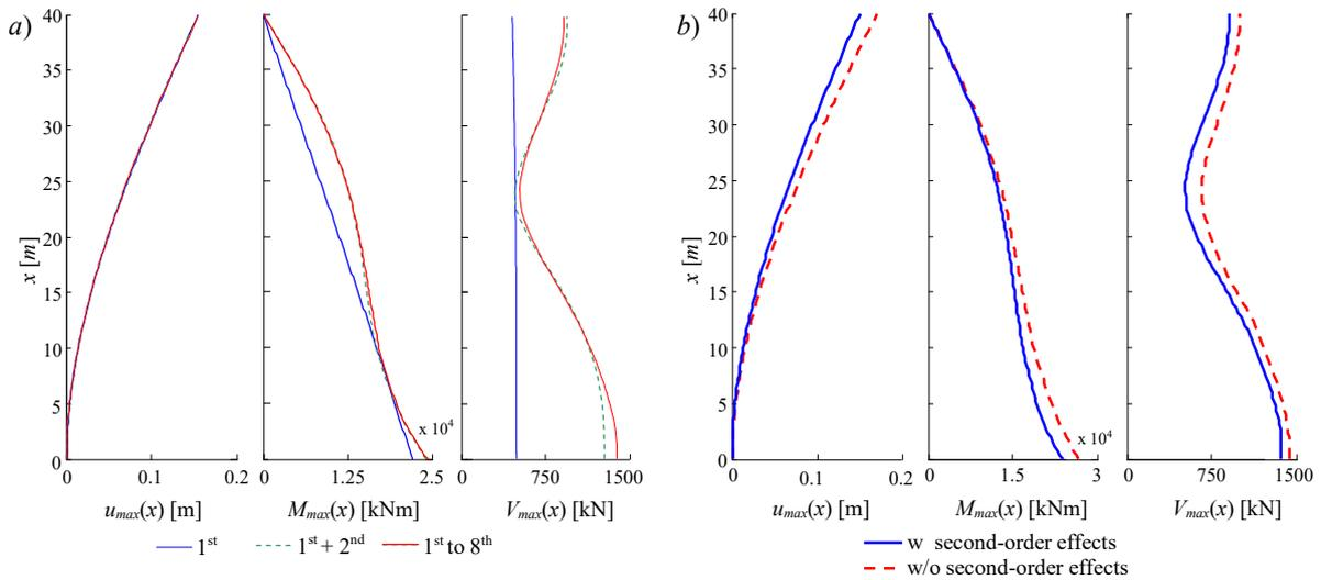
406 Fig. 8 Average seismic response of case study 1: a) modal contributions to the displacements,
