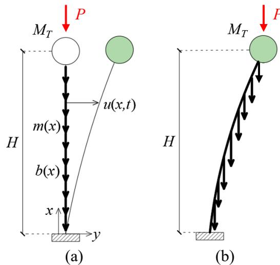
122 Fig. 1. a) Pier model and undeformed configuration; b) deformed pier configuration.
