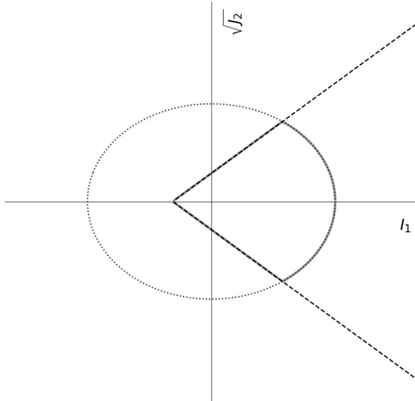
Figure 7: Yield surface (grey solid line) of the capped model  $y_{\text{capped}}$  in the meridional plane, where the black dashed line is the yield surface of the uncapped model  $y_{\text{uncapped}}$  and the black dotted line is the yield surface of the elliptical compressive cap  $y_{\text{cap}_c}$ .
