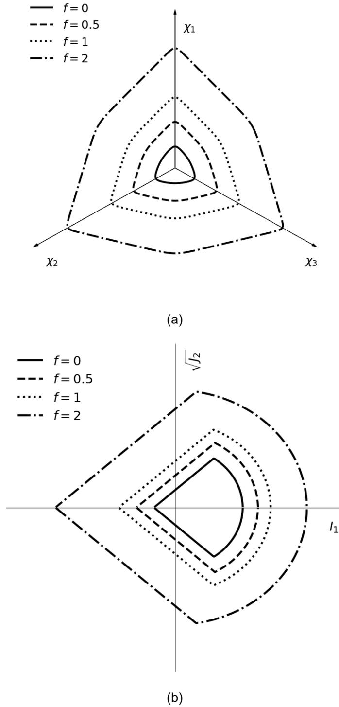
Figure 9: Yield surfaces in the inadmissible stress space (i.e.  $f > 0$ ) for (a) the convex and smooth approximation of the Matsuoka-Nakai yield function (Eq. 26) in the deviatoric plane for  $\phi = \frac{\pi}{6}$ ; (b) the capped yield function (Eq. 30) in the meridional plane.
