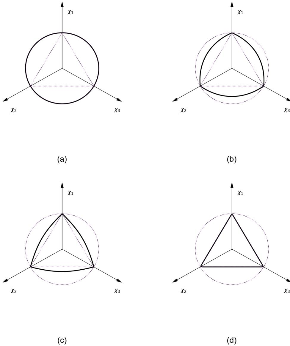
Figure 6: The convex and smooth 'Reuleaux triangle'-shaped yield function defined by Eq. 30 in the deviatoric plane (shown in black solid line) for (a)  $w = 0$  (b)  $w = \frac{1}{3}$  (c)  $w = \frac{2}{3}$  (d)  $w = 1$ . The black dotted lines are the components of the convex combination in Eq. 28.
