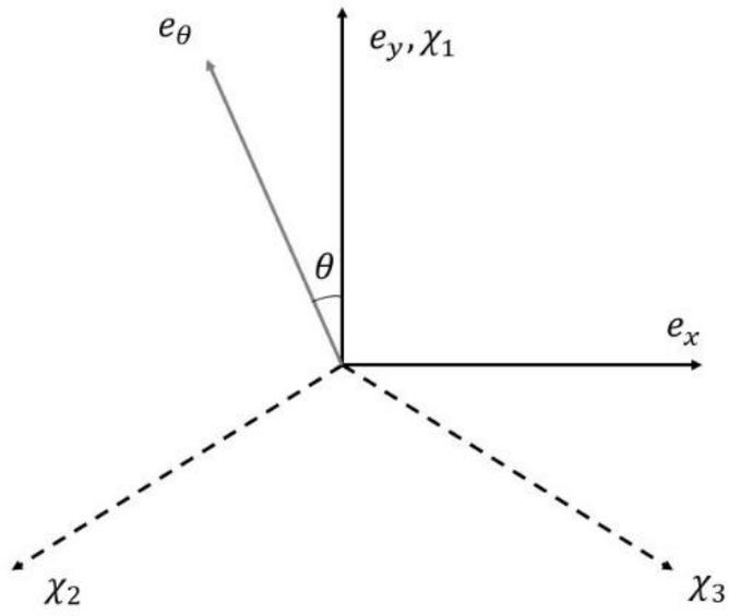
Figure 2: Schematic diagram of a generalised vector  $e_\theta$  that points in any arbitrary direction along the deviatoric plane, where  $\theta$  is the Lode angle.
