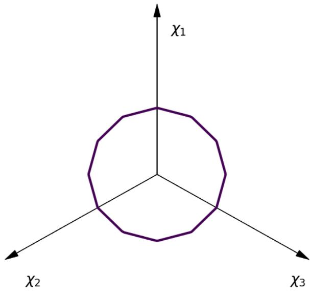
Figure 4: 12-sided polygonal yield surface in deviatoric plane
