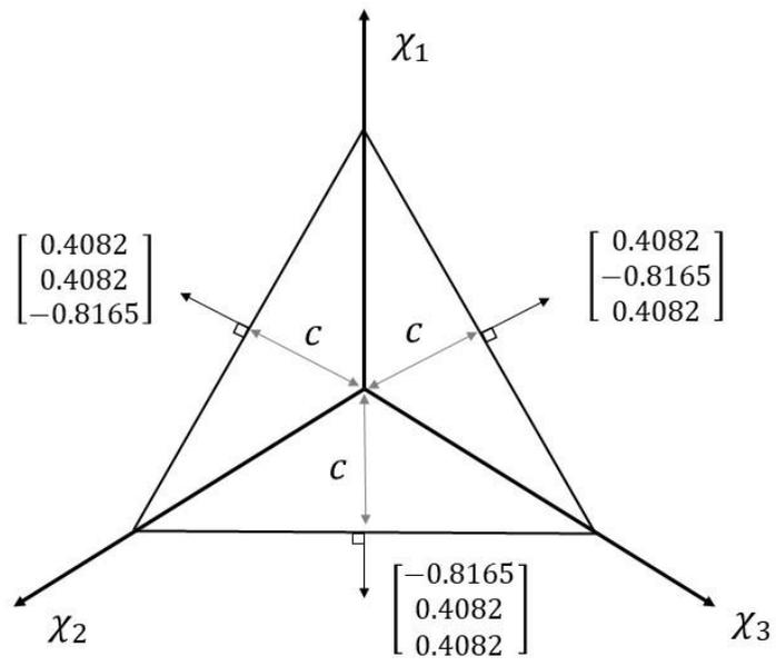
Figure 3: Schematic diagram showing the normal vectors of the hyperplanes that define the 3-sided polygonal yield surface in Eq. 24. Each hyperplane has a projected normal distance of  $c$  from the origin of the stress space.
