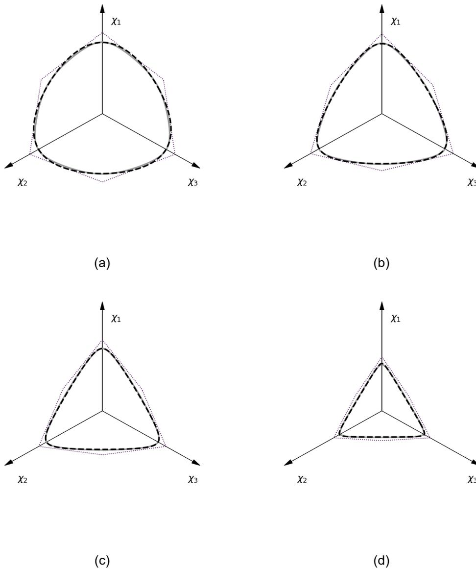
Figure 5: Original Matsuoka-Nakai yield function (black dashed line) and a convex and smooth approximation of the Matsuoka-Nakai yield function (grey solid line) in the deviatoric plane for (a)  $\phi = \frac{\pi}{12}$  (b)  $\phi = \frac{\pi}{6}$  (c)  $\phi = \frac{\pi}{4}$  (d)  $\phi = \frac{\pi}{3}$ . These lines virtually overlap each other. The black dotted line is the 'bounding support function' for the convex and smooth approximation of the Matsuoka-Nakai yield function.
