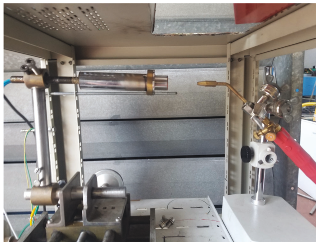
Figure 8: Oxyacetylene torch for convective-radiative heat flux–side view
