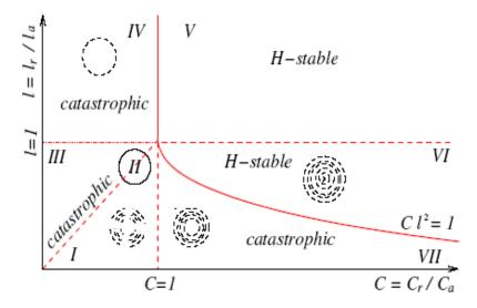
Fig.1. *H*-stability phase diagram of the Morse potential. Catastrophic and stable behaviors are predicted as a function of the parameter ratios  $(I_r/I_a)$  and  $(C_r/C_a)$  [adapted from reference 16]
