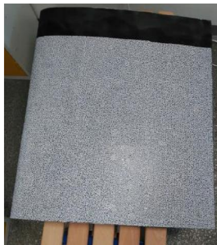
Figure 2 - Speckle pattern applied to solid foil
