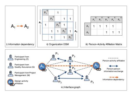
Figure 2. Information inputs for the analysis of process interfaces (generic example): (i) shows the direction of the information dependency between activities  $A_1$  and  $A_2$ ; (ii) shows the organization DSM matrix for people  $P_1$  to  $P_5$ ; (iii) shows the person-activity affiliation matrix; (iv) shows the process interface graph generated as a result of combining (i), (ii), and (iii).
