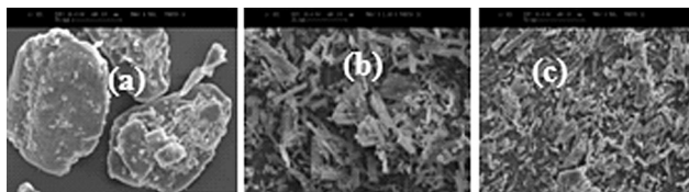
Fig. 1. SEM images for (a) commercial mannitol (b) mannitol crystallised from acetone: water (100:0 ml) and (c) from acetone: water (97.5, 2.5).
