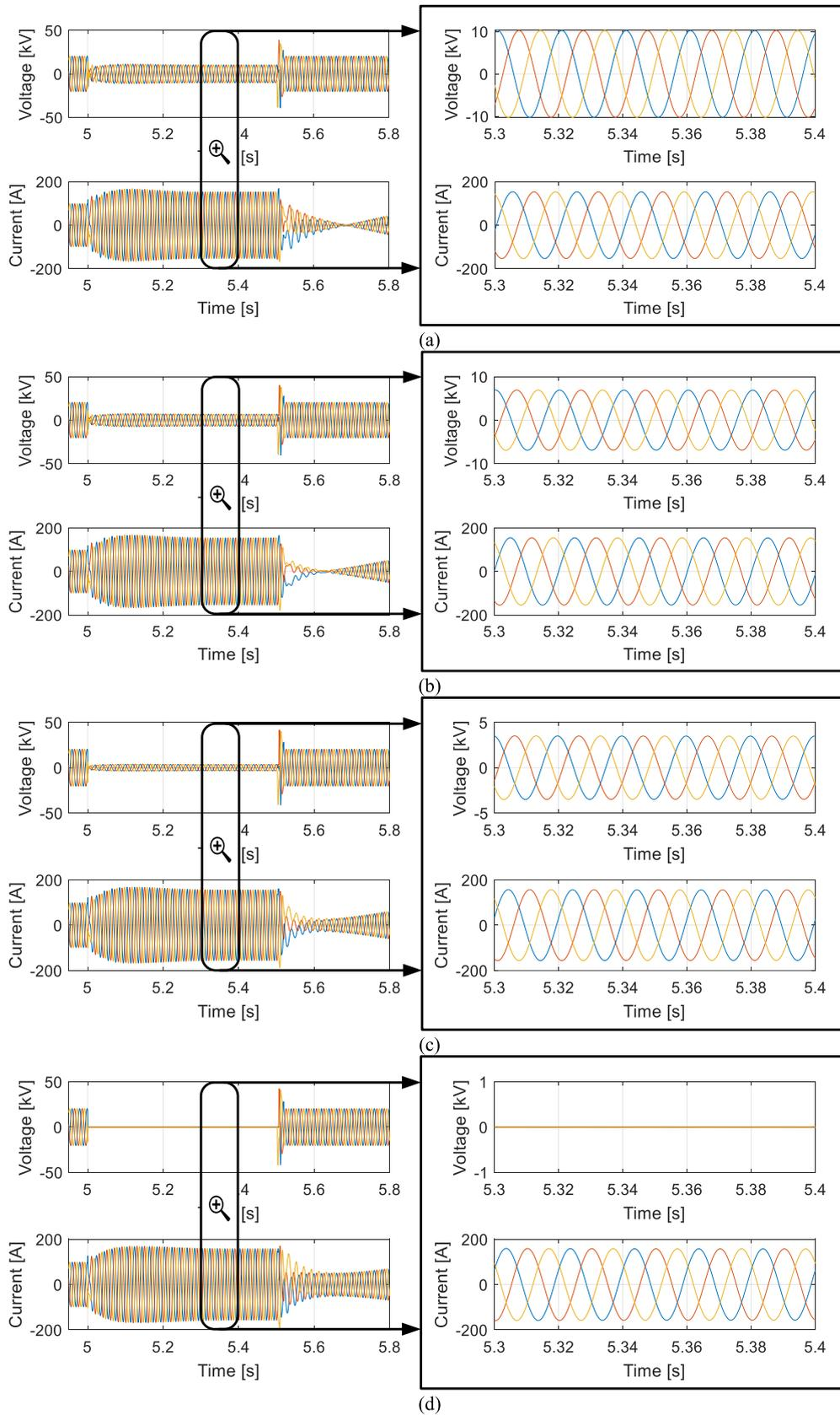
**FIGURE 12.** A three-phase to ground fault was applied at different locations in low SCR, (a)  $FL_4$ , (b)  $FL_3$ , (c)  $FL_2$ , and (d)  $FL_1$ .
