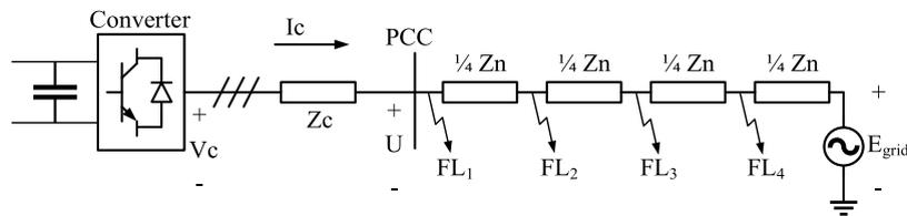
FIGURE 10. Fault locations used in the first analysis.
