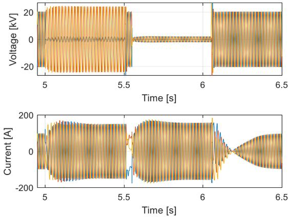
FIGURE 15. Unbalanced fault followed by a balanced fault in high SCR.
