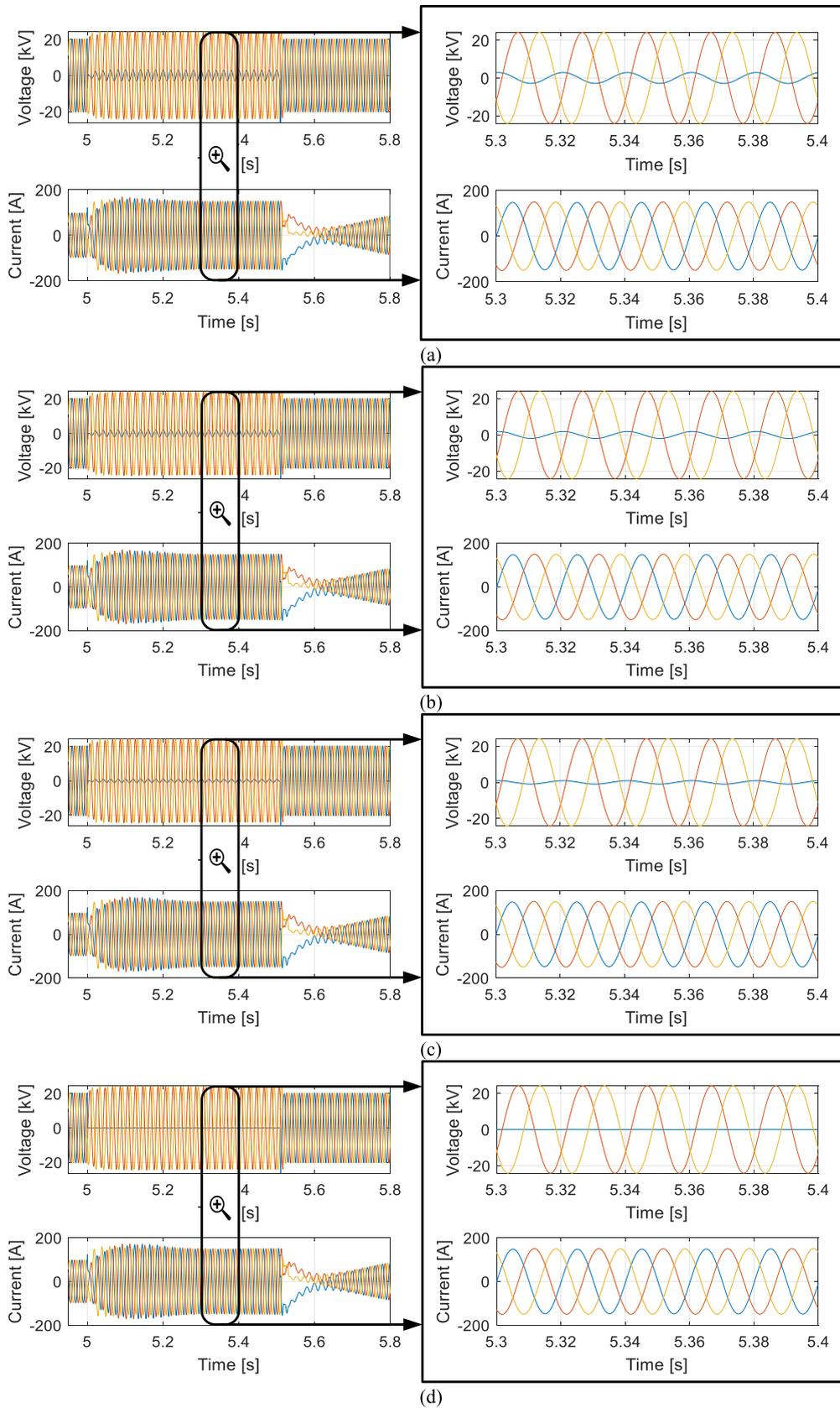
**FIGURE 13.** A single-phase to ground fault results at different locations with high SCR, (a) FL<sub>4</sub>, (b) FL<sub>3</sub>, (c) FL<sub>2</sub>, and (d) FL<sub>1</sub>.
