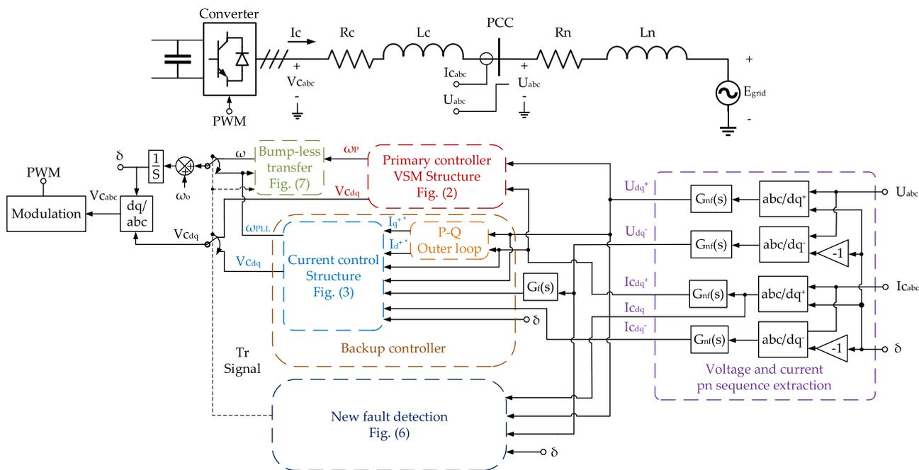
FIGURE 5. A full schematic of the improved dual VSM structure. outer loop (orange), bump-less transfer (green), new FDA (dark blue).
