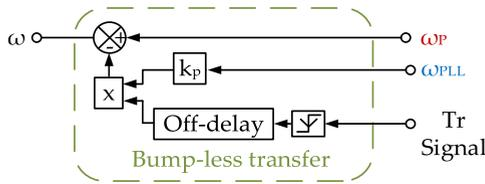
FIGURE 7. Bump-less transfer activated during fault recovery.
