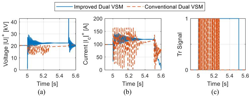
FIGURE 9. Comparison between improved dual VSM and conventional dual VSM in the low SCR case.
