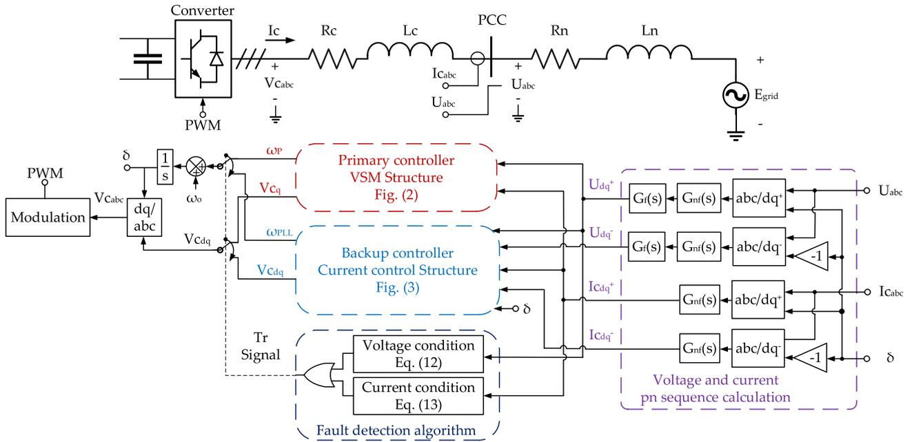
**FIGURE 1.** Dual VSM structure. (purple) positive and negative voltage and current calculation, VSM structure (red), current control structure (blue), and fault detection algorithm (navy).
