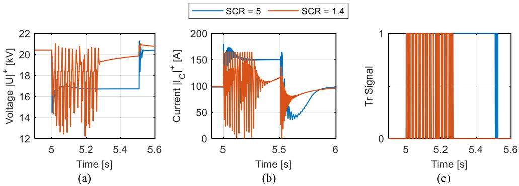
**FIGURE 4.** Comparison in low SCR (1.4) and high SCR (5), (a) positive sequence voltage magnitude  $|U|^+$  at the PCC, (b) positive sequence current magnitude  $|I_c|^+$ , (c) FDA output signal (Tr signal).
