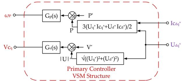
**FIGURE 2.** Schematic of the primary controller (VSM structure).
