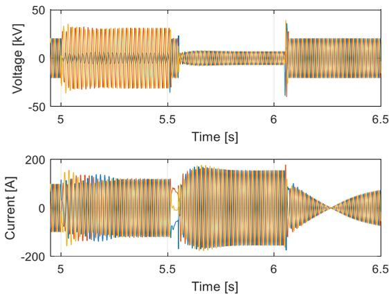
FIGURE 16. Unbalanced fault followed by a balanced fault in low SCR.
