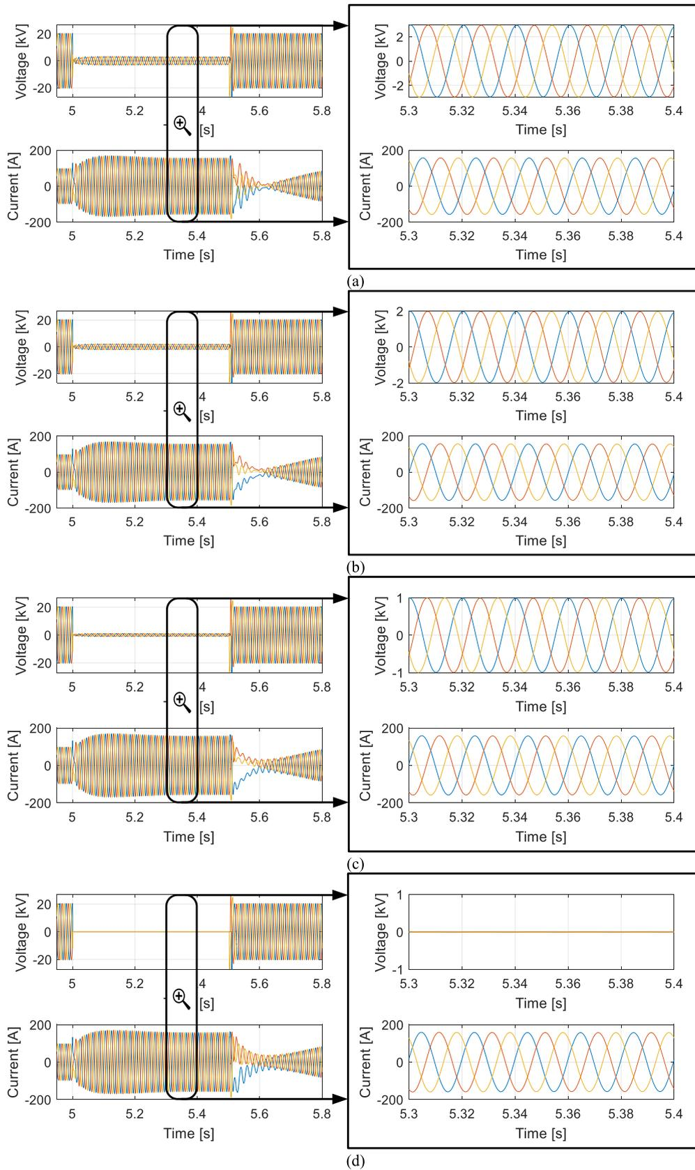
**FIGURE 14.** A three-phase to ground fault was applied at different locations in high SCR, (a)  $FL_4$ , (b)  $FL_3$ , (c)  $FL_2$ , and (d)  $FL_1$ .
