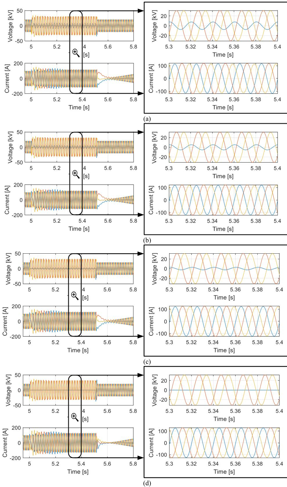
**FIGURE 11.** A single-phase to ground fault results at different locations in low SCR, (a) FL<sub>4</sub>, (b) FL<sub>3</sub>, (c) FL<sub>2</sub>, and (d) FL<sub>1</sub>.
