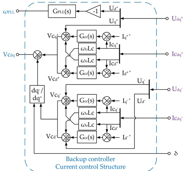
FIGURE 3. Schematic of the backup controller (pn sequence CC).
