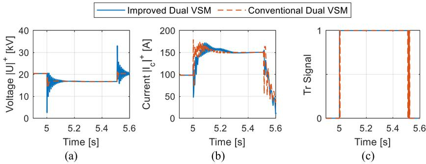
FIGURE 8. Comparison between improved dual VSM and conventional dual VSM in the high SCR case.
