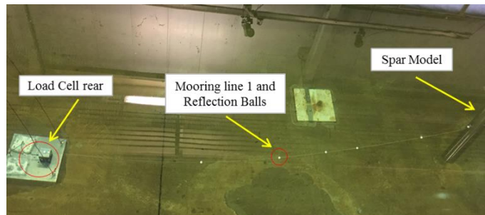
Figure 11 Mooring line with underwater reflection balls in the tank
