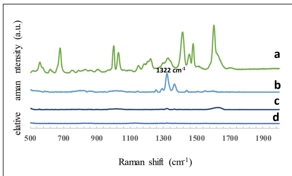
**Figure 1:** Raman spectra of solid warfarin (a) and (b) representative SERS spectra of warfarin standard solutions using PDDA coated Ag NPs at concentrations of 36 nM warfarin, (c) 1.9  $\mu\text{M}$  warfarin solution and (d) the colloid substrate solution only. Laser excitation at 638 nm and integration time = 20 s. Spectra have been vertically offset for clarity.
