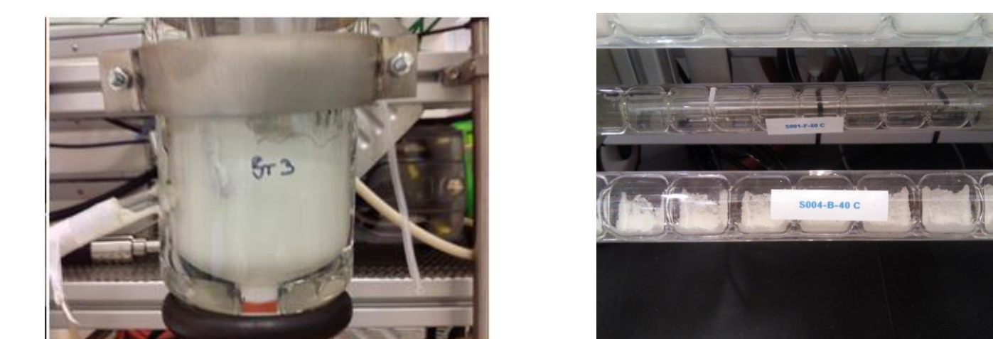
Fig. 12: Images showing extent of encrustation in COBC and MSMPR reactor vessel.
