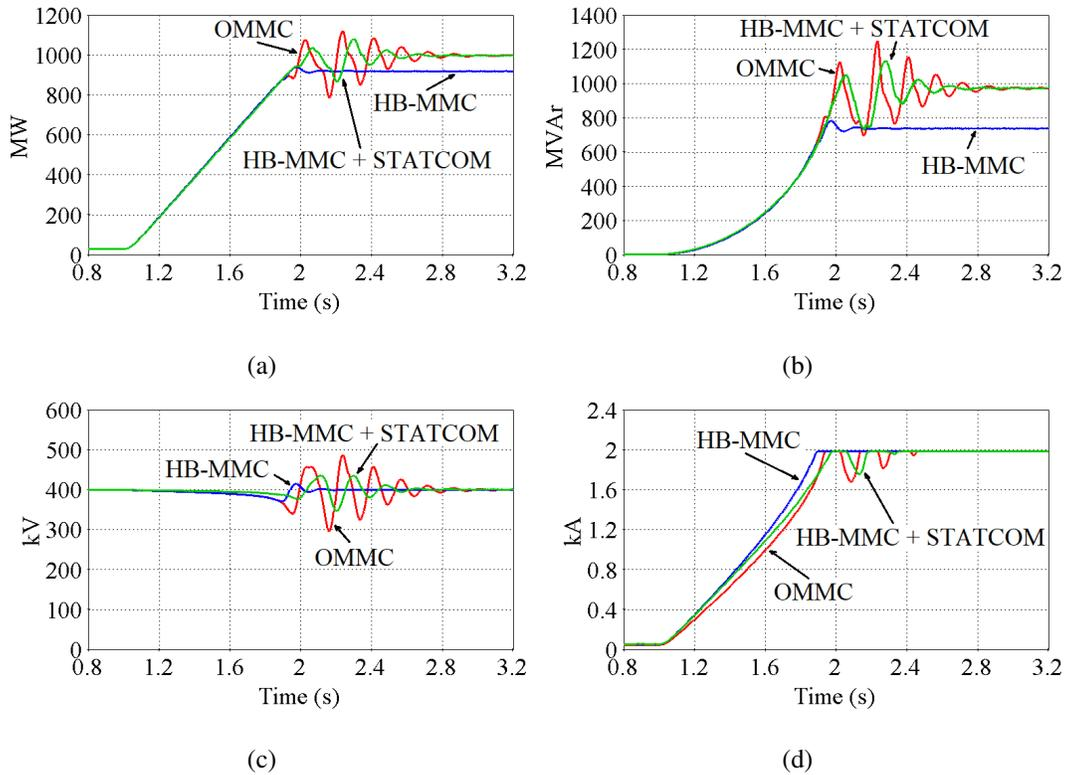
Figure 19: Expansion of the PQ capability in a weak network (a) Active power, (b) Reactive power, (c) Grid RMS voltage, (d) Converter RMS current.
