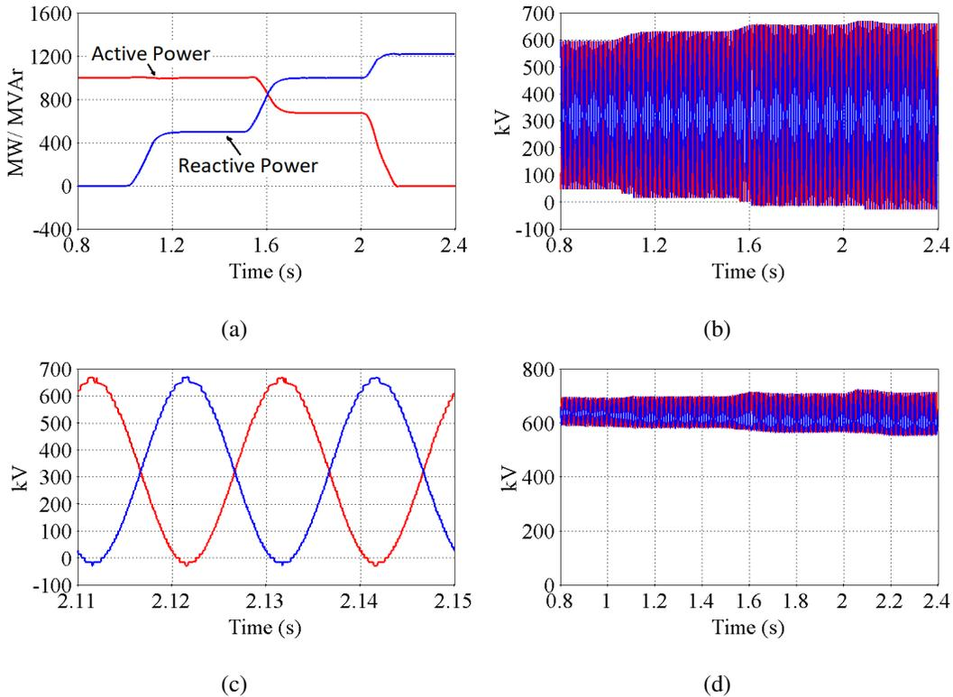
Figure 18: Expansion of the PQ capability (a) Active and Reactive power, (b) Arm voltages, (b) Focused arm voltages, (d) Total capacitor voltages.
