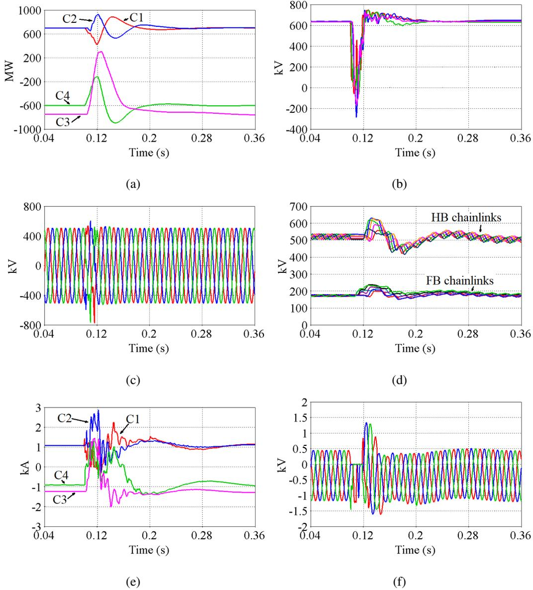
Figure 15: Illustrative operation of a four terminal system (a) Active powers, (b) DC voltages, (c) Converter 1 AC side voltages, (d) Converter 1 Capacitor voltages, (e) DC currents, (f) Converter 1 upper arm currents.
