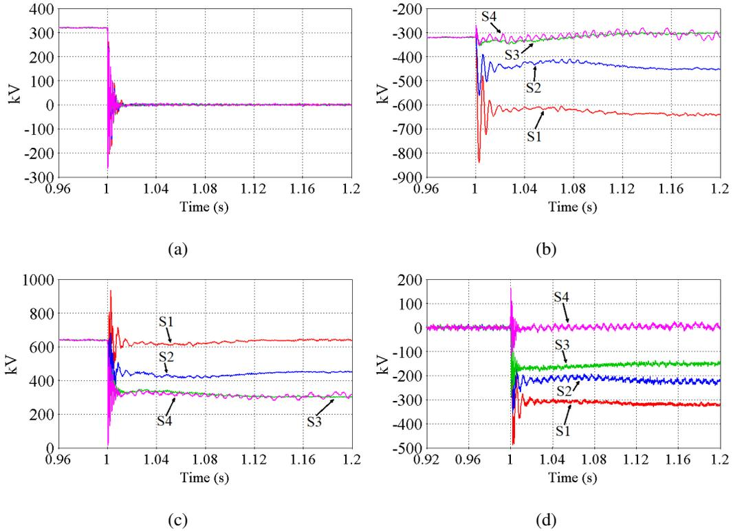
Figure 6: P2G DC fault simulation waveforms for cases highlighted in Table 2: (a) positive pole-to-ground DC voltage (faulty pole), (b) negative pole-to-ground voltage (healthy pole), (c) pole-to-pole DC voltage, (d) DC voltage stresses on the interfacing transformer.
