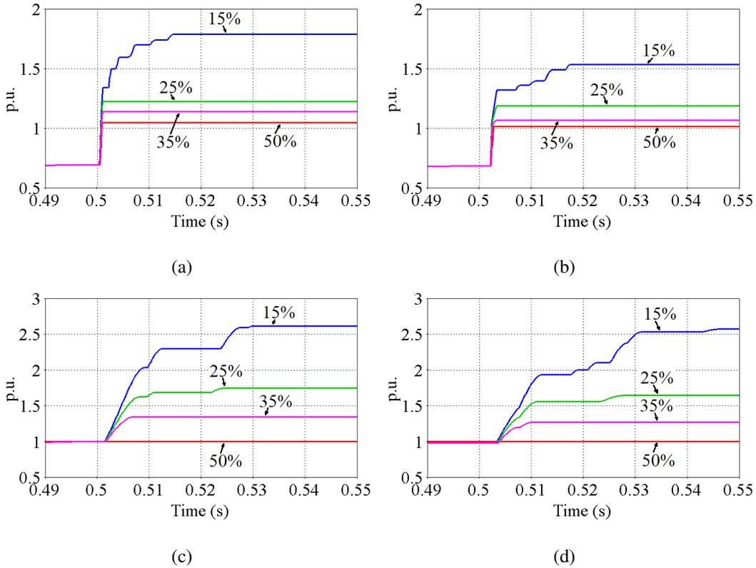
Figure 8: The effect of constant various ratio of FB cells during DC fault with rectified HB cells (a) Maximum values of arm currents of converter 1, (b) Maximum values of arm currents of converter 2, (c) Maximum values of cell voltages of converter 1, (d) Maximum values of cell voltages of converter 2.
