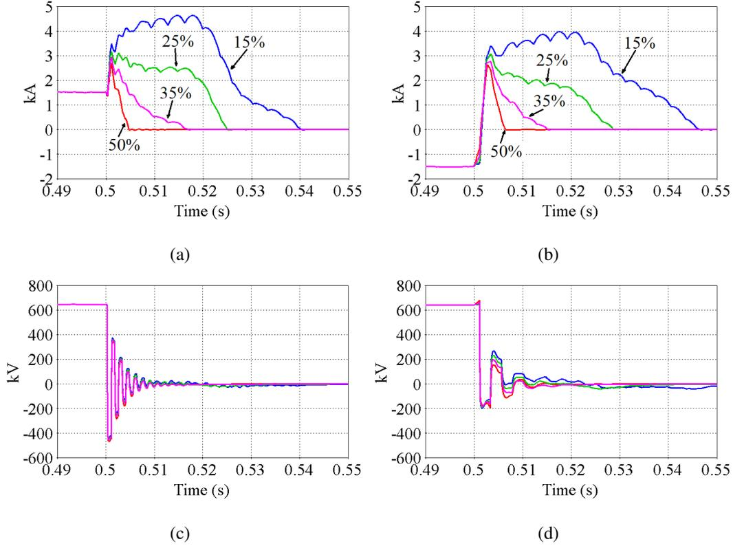
Figure 10: DC voltages and currents for different FB ratios with rectified HB cells (a) DC currents converter 1, (b) DC currents converter 2, (c) DC voltage converter 1, (d) DC voltage converter 2.
