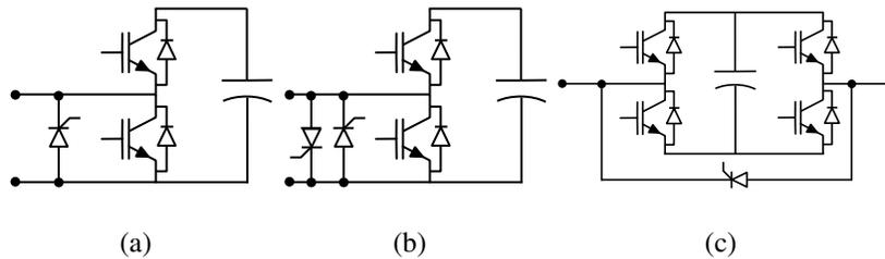
Figure 4: Cell topologies with bypass thyristors (a) HB cell with single bypass thyristor, (b) HB cell with back-to-back thyristor, (c) FB cell.
