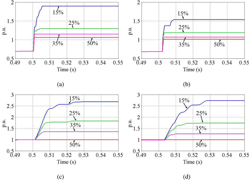
Figure 11: The effect of constant various ratio of FB cells during DC fault with fully bypassed HB cells (a) Maximum values of arm currents of converter 1, (b) Maximum values of arm currents of converter 2, (c) Maximum values of cell voltages of converter 1, (d) Maximum values of cell voltages of converter 2.
