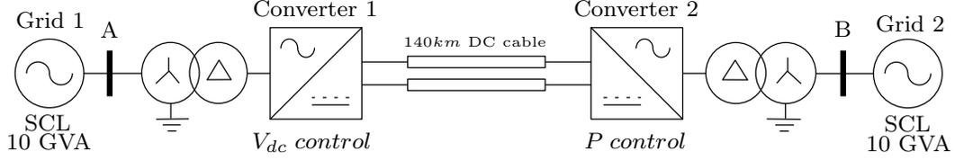
Figure 5: Simulated DC network.
