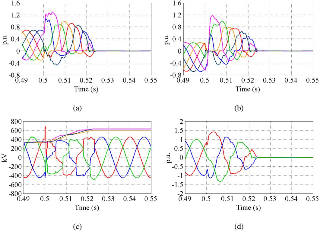
Figure 12: Arm currents during the DC fault for different FB ratios with fully bypassed HB cells (a) 50% FB ratio converter 1, (b) 50% FB ratio converter 2, (c) 25% FB ratio converter 1, (d) 25% FB ratio converter 2, (e) AC Line-to-Line voltage superimposed with the FB cell voltages, (f) Converter side AC currents.
