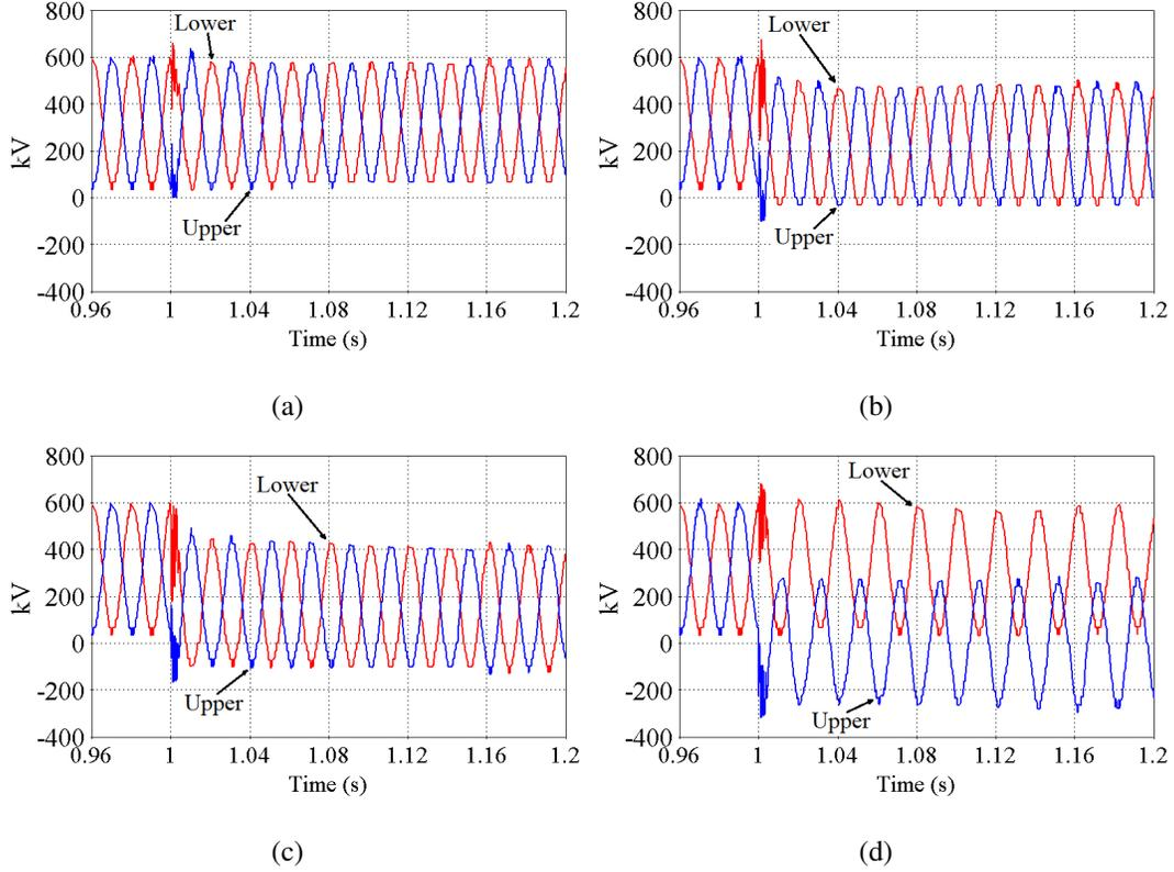
Figure 7: Arm voltages during P2G DC fault for cases highlighted in Table 2: (a) 0% CMMC (HB-MMC), (b) 15% CMMC at 0.7 pu DC voltage adjustment, (c) 25% CMMC at 0.5 pu DC voltage adjustment, (d) 50% CMMC (MC-MMC) at 0.5 pu DC voltage adjustment.
