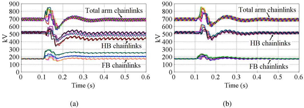
Figure 17: The effect of horizontal controller under disturbance on the capacitor voltages (a) Conventional, (b) Modified. C2, DC currents of converters C1 to C4 and arm currents of C2, originally displayed in Fig. 15. These expanded plots confirm the effectiveness of the CMMC in driving down the faults currents in AC and DC sides, where the converters' semiconductors and DCCBs are affected.
