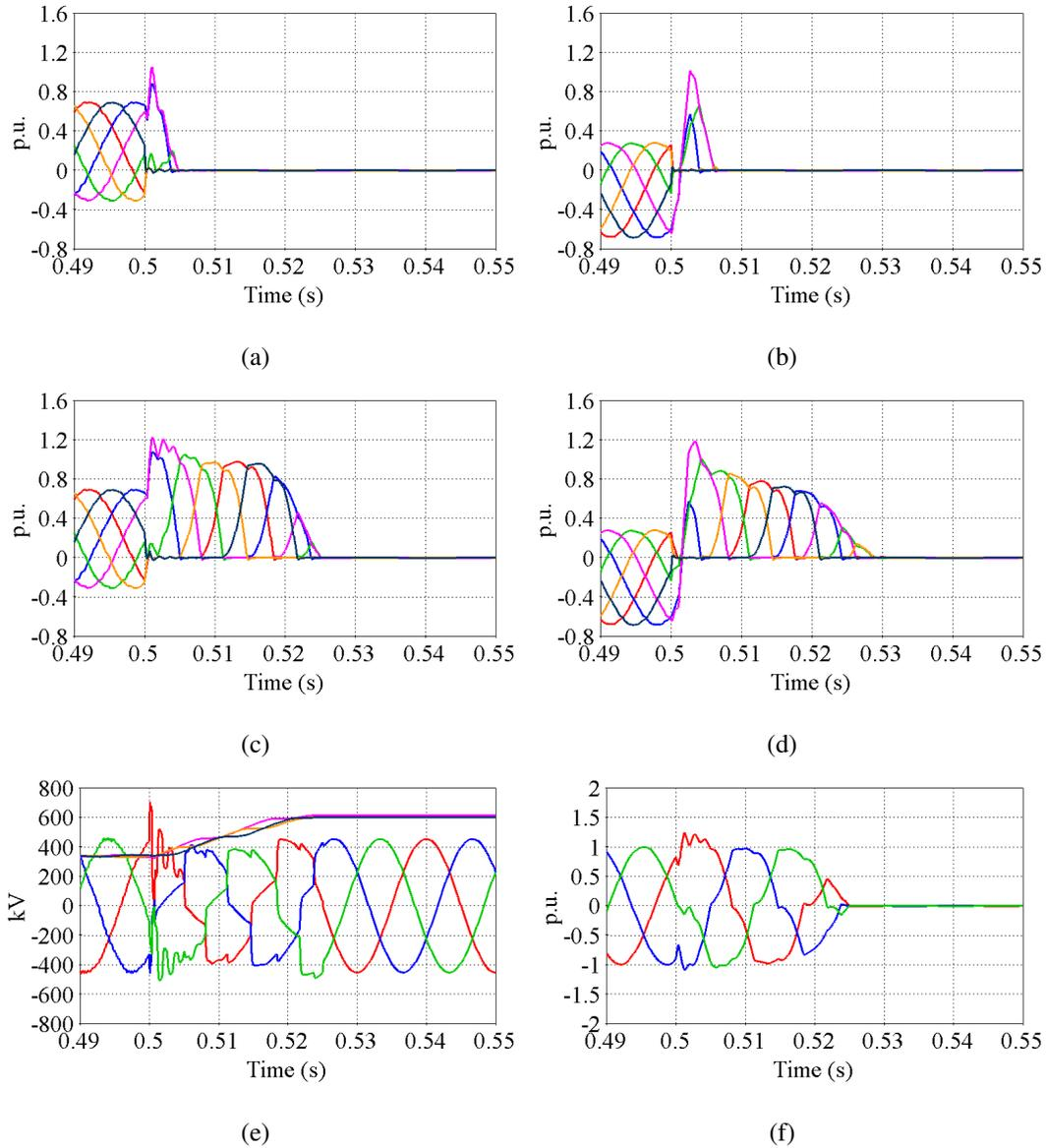
Figure 9: Arm currents during the DC fault for different FB ratios with rectified HB cells (a) 50% FB ratio converter 1, (b) 50% FB ratio converter 2, (c) 25% FB ratio converter 1, (d) 25% FB ratio converter 2, (e) AC Line-to-Line voltage superimposed with the FB cell voltages, (f) Converter side AC currents.
