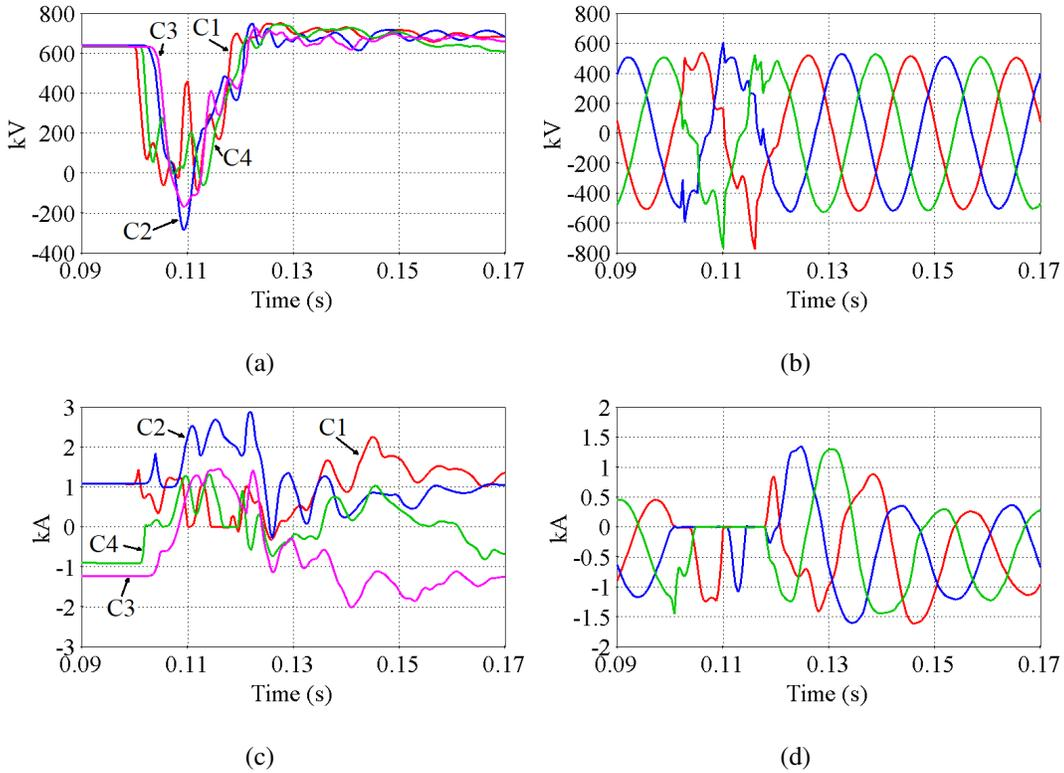
Figure 16: Focused illustrative operation of a four terminal system (a) DC voltages, (b) Converter 1 AC side voltages, (c) DC currents, (d) Converter 1 upper arm currents.
