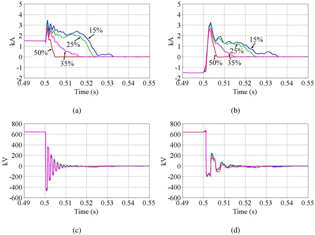
Figure 13: DC voltages and currents for different FB ratios with fully bypassed HB cells (a) DC currents converter 1, (b) DC currents converter 2, (c) DC voltage 1, (d) DC voltage converter 2.
