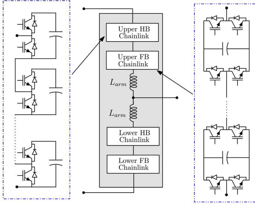
Figure 1: Multilevel HVDC converter topologies.
