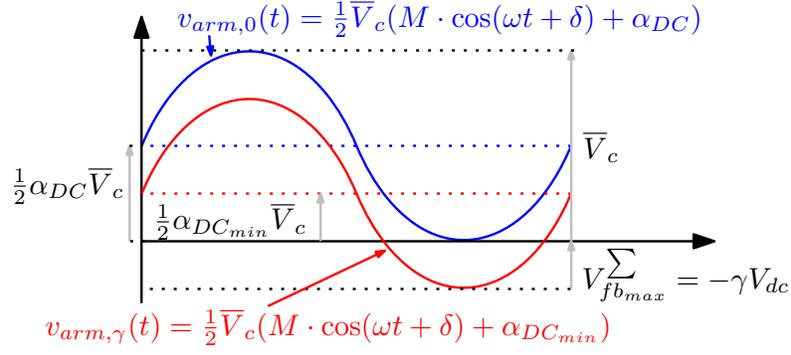
Figure 2: Arm modulation signals of CMMC.
