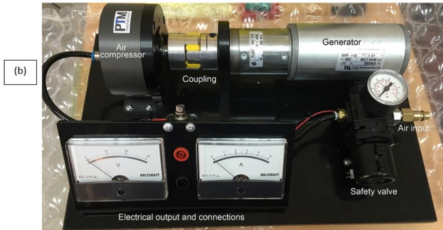
Figure 9: (a) System diagram of a micro-CAES (b) Prototype of micro-CAES [133]
