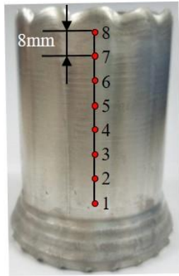
Fig. 14. Wall-thickness measuring points along the axial direction.
