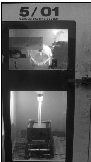
Fig 19: Vacuum casting Impeller
