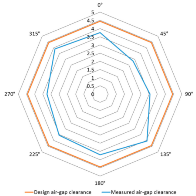
Figure 4. Airgap clearance (in mm) for the Northern Power 1.5MW prototype. The values shown here are the mean of the airgap clearance at the upwind and downwind ends of the machine. Clearance is plotted for different angles as seen from the upwind end of the machine. (This figure is available in colour online.)
