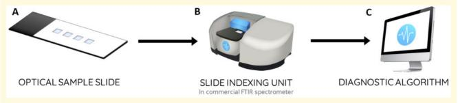
Figure I The spectroscopic liquid biopsy platform. (A) Optical sample slides containing four wells, for triplicate sample measurements and a single background measurement; (B) slide indexing unit to integrate slides with a commercially available FTIR spectrometer; and (C) diagnostic algorithm contained within bespoke operating software that auto-generates a disease prediction.
