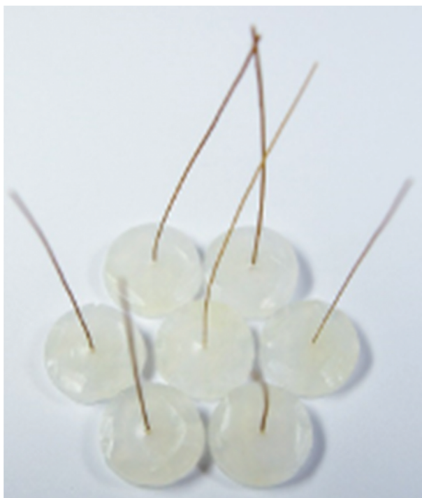
Figure 8. Example of typical Coir-PP cylindrical pull-out samples.
