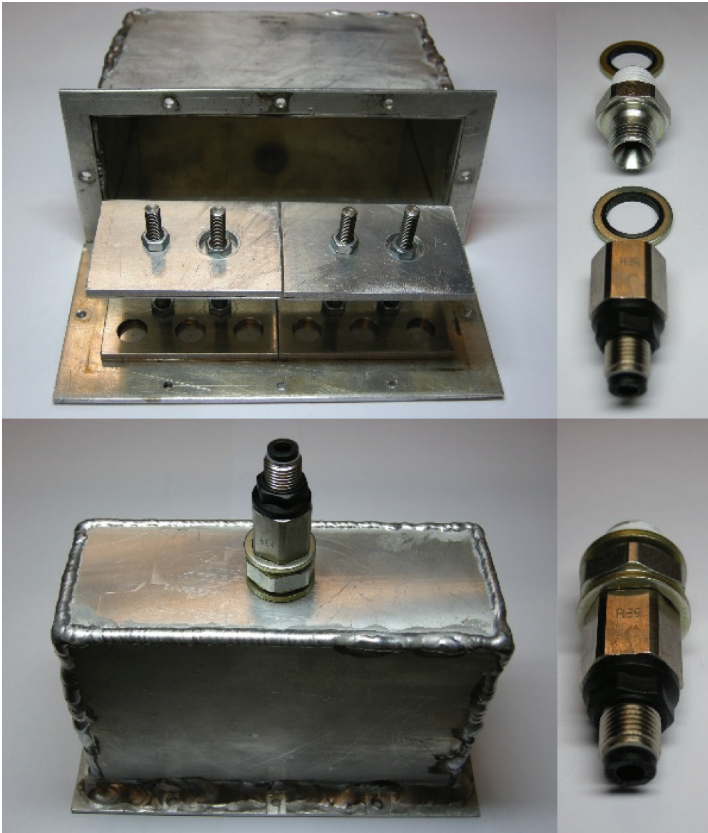
Figure 5. Metal frame and chamber with the gas connection.
