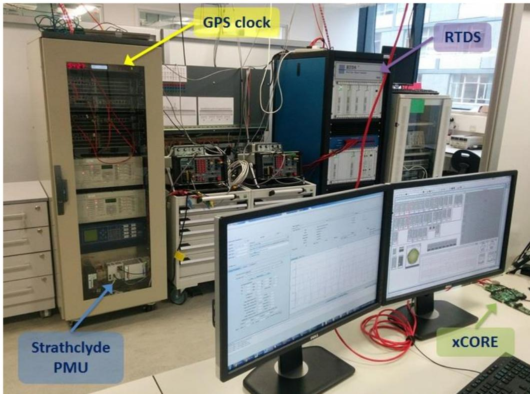
Figure 5: Laboratory testing configuration
