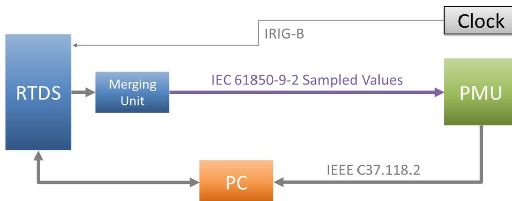
Figure 4: PMU testing using IEC 61850-9-2 SV protocol
