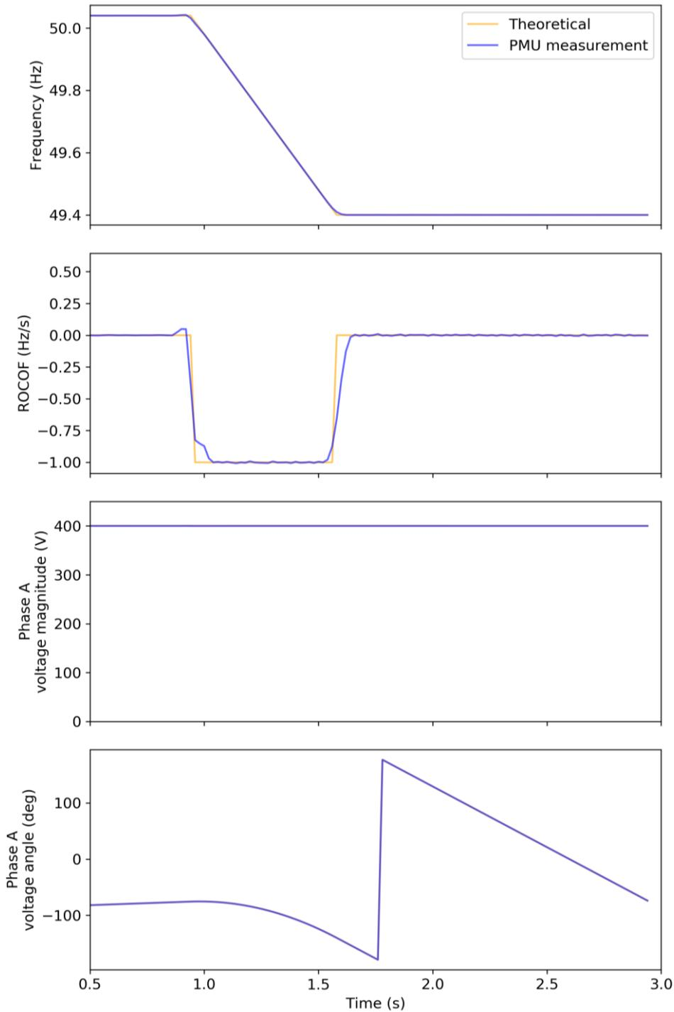
**Figure 9: Comparison of theoretical and measured parameters**
