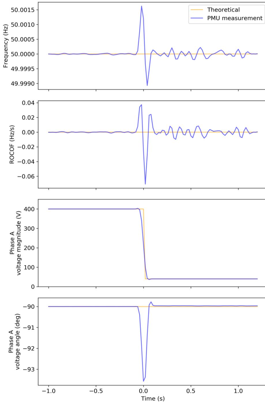
**Figure 10: Comparison of theoretical and measured parameters during emulated fault**
