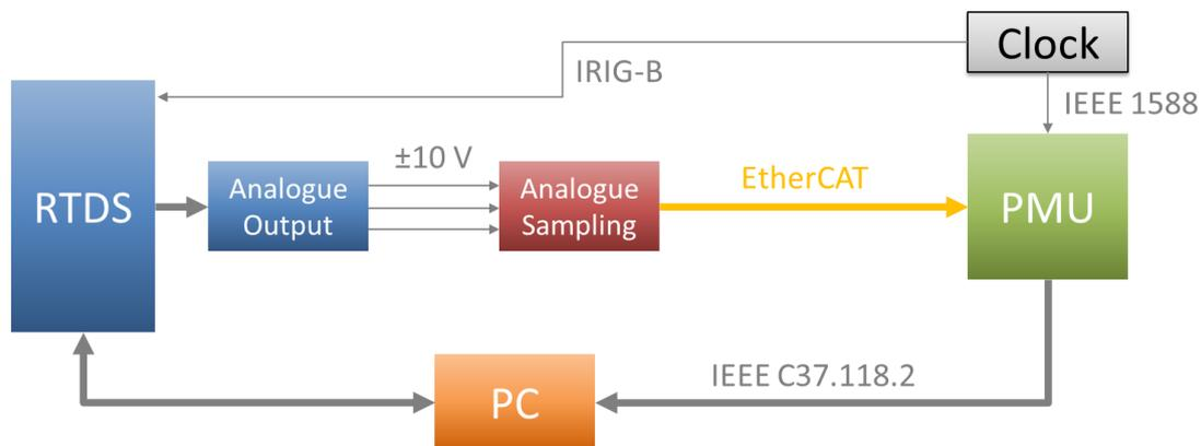
Figure 3: PMU closed-loop testing configuration
