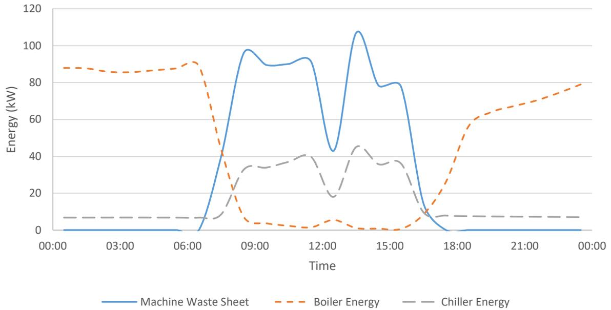
Figure 4- Waste heat output from machinery alongside energy required for boiler and chiller systems
