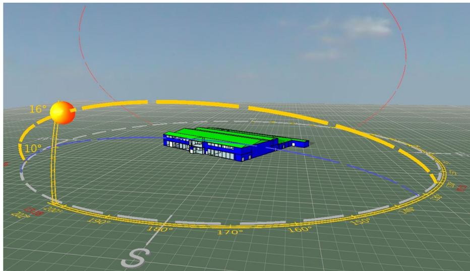
Figure 2- Building model in IES-VE, displaying the solar path around the building
