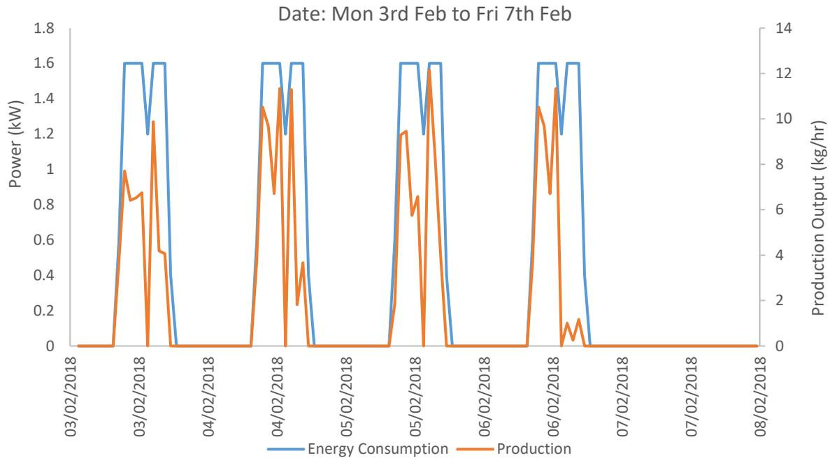
Figure 7 - Energy Use VS Production Output for Bumotec Turnmill
