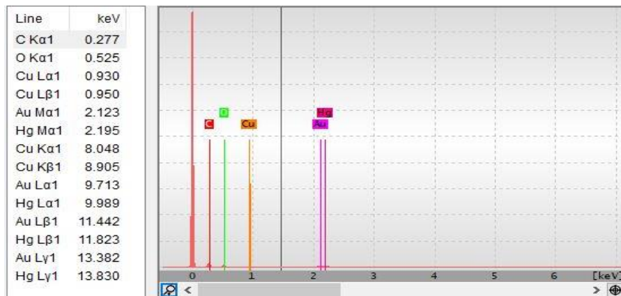
Figure 2: SEM images of (a) TMCC (micocrystalline cellulose (MMC) modified with 1, 2, 3, 4-butanetetracarboxylic acid (BTCA)). (a) TMCC loaded with Pb(II) ions, respectively; (c) associated energy-dispersive X-ray analysis (EDX) patterns for TMCC and TMCC loaded with Hg(II) ions.
