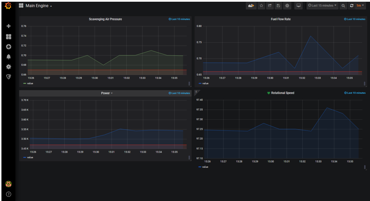
Figure 4. Data dashboard of four main engine parameters in Grafana.
