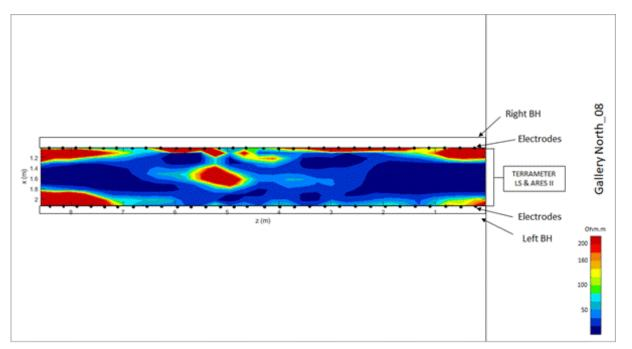
Figure 2: Cross borehole Survey S2 (RMS = 12.7%)
