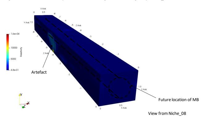
Figure 4: 3D view of inversion results from survey T1 (RMS = 10.7%)
