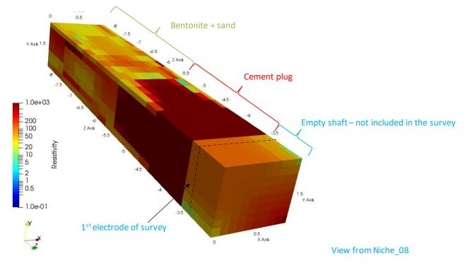
Figure 6: 3D view of inversion results from survey T2 (RMS = 5.16%)
