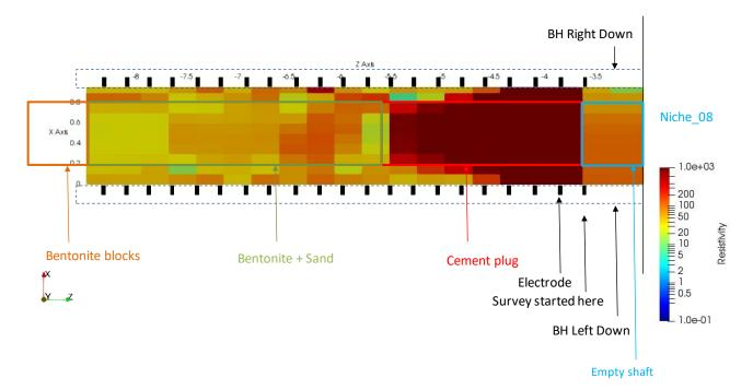
Figure 7: Cross section view of inversion results from survey T2 (RMS = 5.16%)
