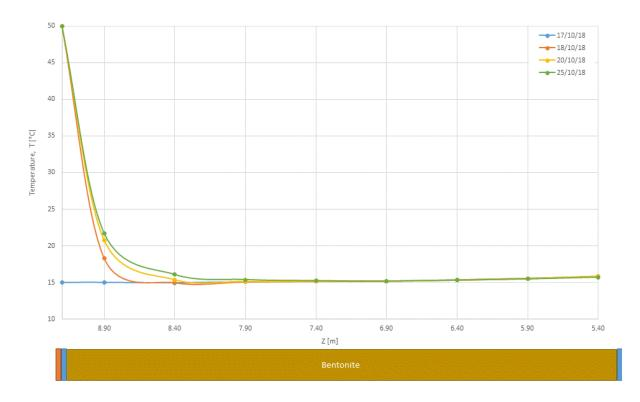
Figure 9: Temperature evolution recorded by temperature sensors installed along the buffer.
