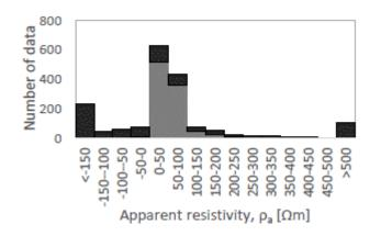
Figure 8: Distribution of apparent resistivity before and after filtering out measurements associated with large geometric factors (black and grey bars, respectively) for survey S2.
