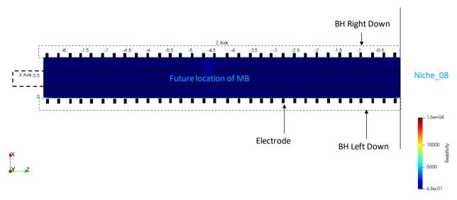
Figure 5: Cross section view of inversion results from survey T1 (RMS = 10.7%)
