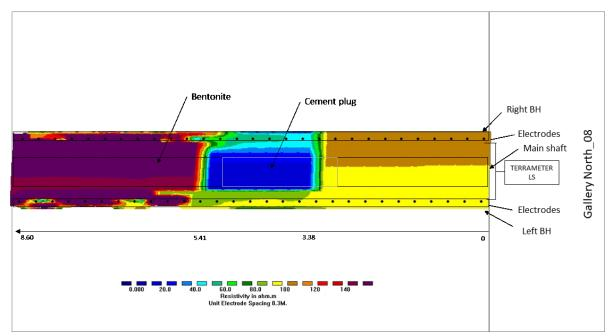
Figure 3: Cross borehole survey S6 (RMS = 1.1%)
