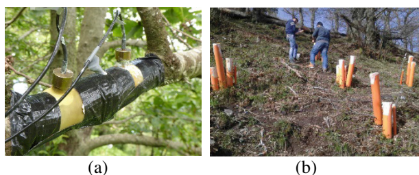
Fig. 2. Soil and plant monitoring at Monte Faito, Naples. (a) High-capacity tensiometers installed on chestnut. (b) Installation of TDR probes and conventional tensiometers in the ground (12/04/2018).
