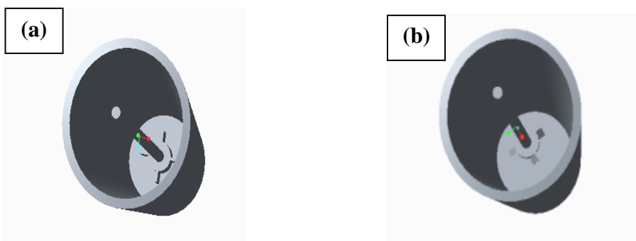
Fig.2 Geometrical model of Crucible with stirrer (a) Crucible with 90^\circ stirrer blade (b) Crucible with 45^\circ stirrer blade
