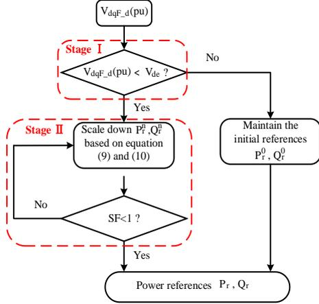
Fig. 3 Flowchart of the designed fault current limiter.
