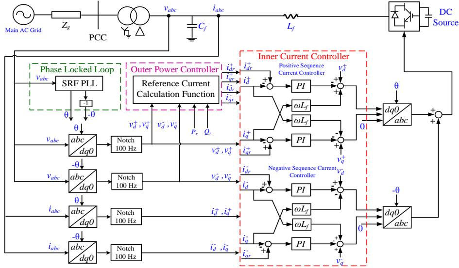
Fig. 2 Control structure of the HVDC system with dual-sequence current control loop [11].
