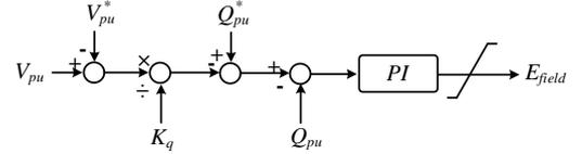
Fig. 5 Structure of the reactive power droop controller.
