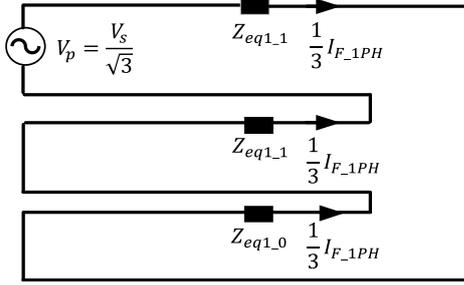
Fig. 6 Sequence network for single phase to ground fault.
