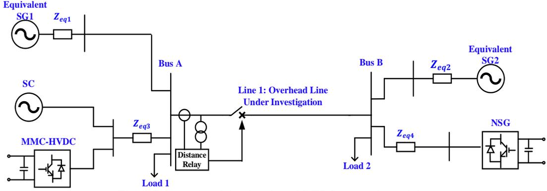
Fig. 1 Schematic of the developed RTDS network model.
